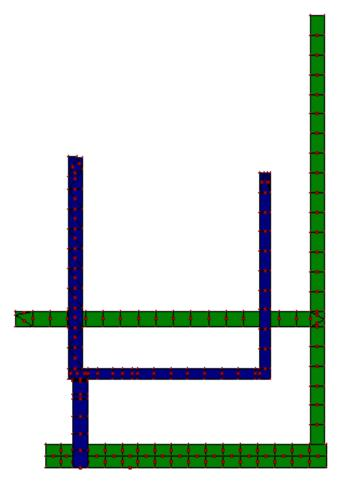
Figure 9. Current distribution of the proposed antenna.
