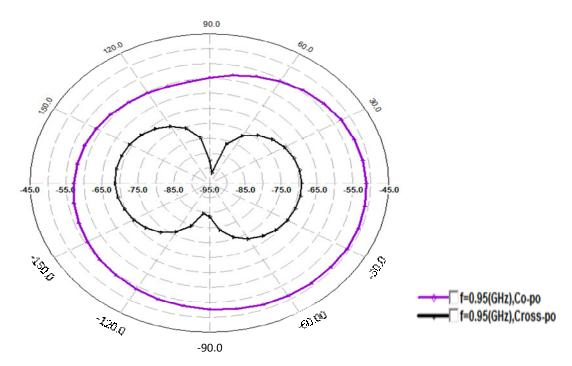
Figure 6b. Azimuth pattern gain display at 90°.
