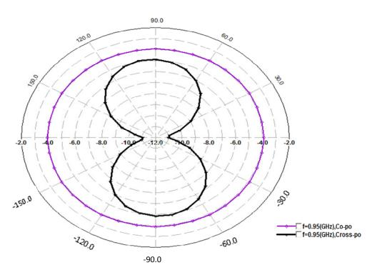
Figure 6a. Azimuth pattern gain display at 0°.
