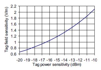
**Figure 2.** Tag field sensitivity (V/m) vs. tag power sensitivity (dBm), frequency is 915 MHz. Source: (Nikitin and Rao, 2008).
