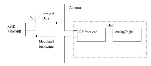
Figure 1. RFID system operation; Source: (Yu et al., 2006).
