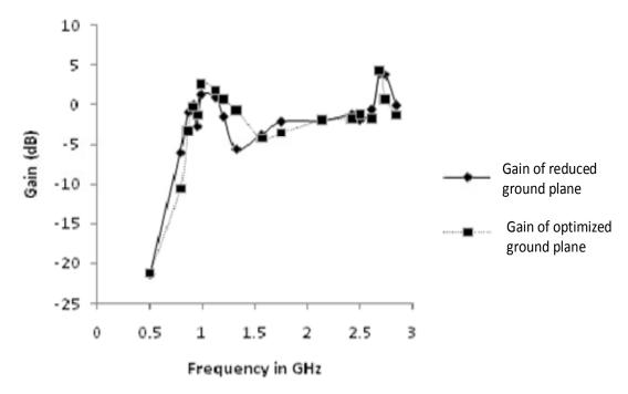
Figure 8. Change in gain as a result of change in ground plane.
