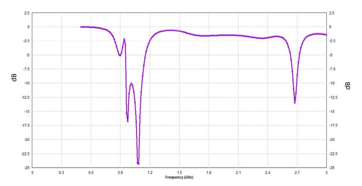
Figure 5. Return loss of the proposed wide slot MSA.
