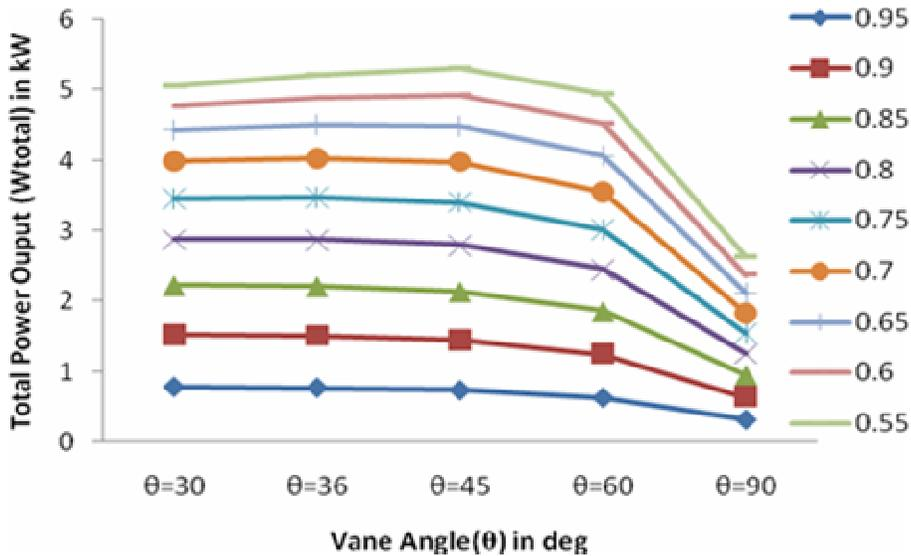
Figure 5. Total power output versus vane angles with respect to rotor / casing diameter (d/D) ratio when D = 100 mm.
