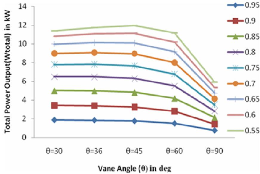
**Figure 6.** Total power output versus vane angles with respect to rotor / casing diameter ( $d/D$ ) ratio when  $D = 150$  mm.
