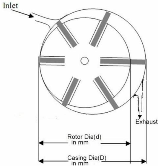
Figure 1a. Air turbine-schematic model.
