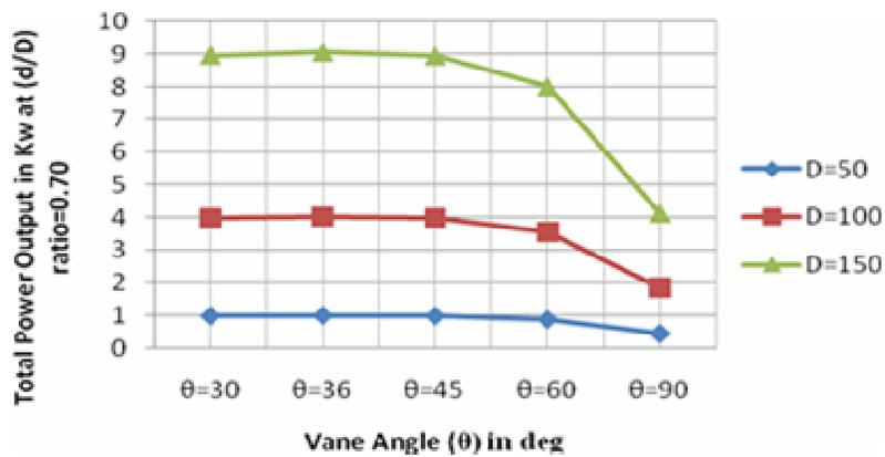
**Figure 8.** Total power output versus vane angles when rotor / casing diameter (d/D) ratio is 0.70 and D = 50, 100 and 150 mm.
