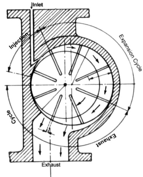
Figure 1b. Air turbine-model.
