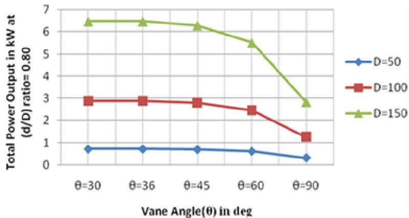
**Figure 9.** Total power output versus vane angles when rotor / casing diameter (d/D) ratio is 0.80 and D = 50, 100 and 150 mm.
