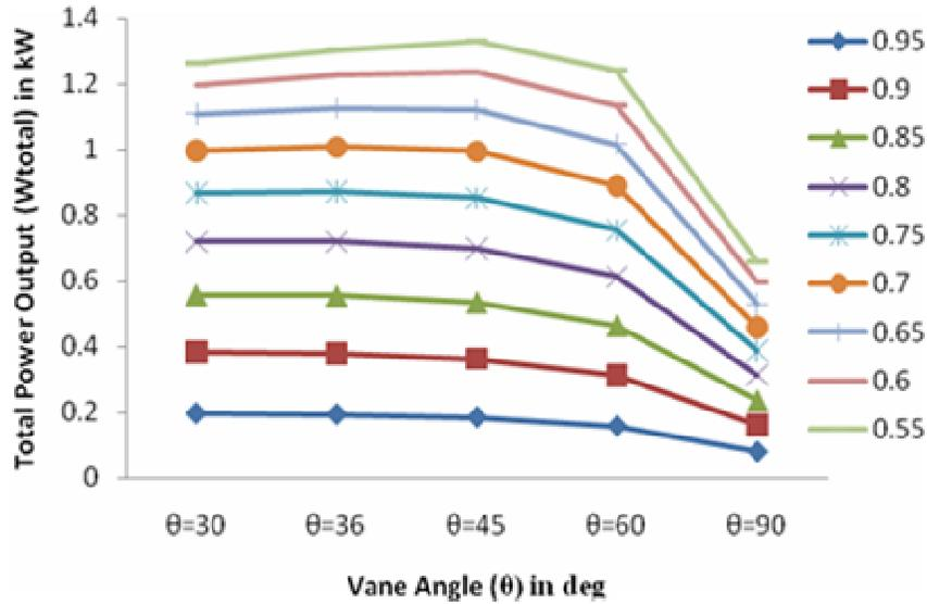
Figure 4(e). Total power output versus vane angles with respect to rotor / casing diameter (d/D) ratio when D= 50 mm.
