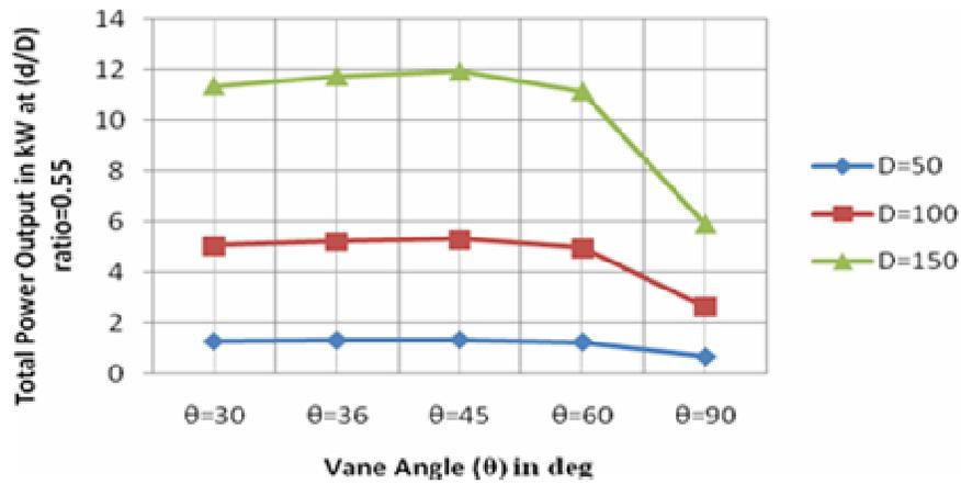
**Figure 7.** Total power output versus vane angles when rotor / casing diameter (d/D) ratio is 0.55 and D = 50, 100 and 150 mm.
