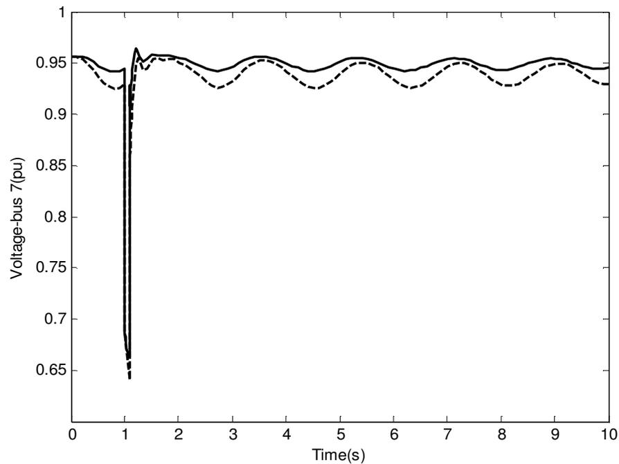
**Figure 11.** Voltage of bus number 7 under scenario 2 in heavy load condition. Solid (with UPFC); Dashed (without UPFC).
