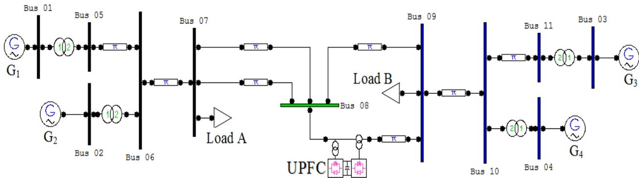
Figure 1. Four-machine eleven-bus power system.
