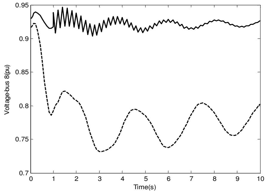
**Figure 6.** Voltage of bus number 8 under scenario 1 in heavy load condition. Solid (with UPFC); Dashed (without UPFC).
