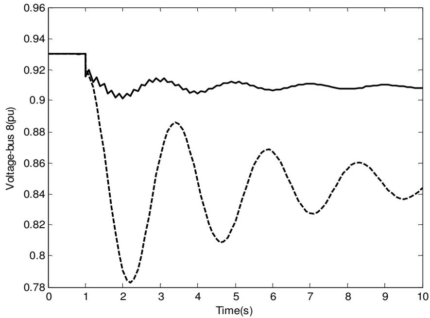
**Figure 4.** Voltage of bus number 8 under scenario 1 in nominal load condition. Solid (with UPFC); Dashed (without UPFC).
