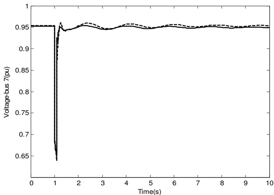
**Figure 9.** Voltage of bus number 7 under scenario 2 in nominal load condition. Solid (with UPFC); Dashed (without UPFC).
