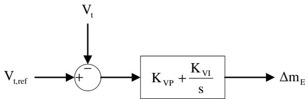
**Figure 3.** Bus voltage controller.
