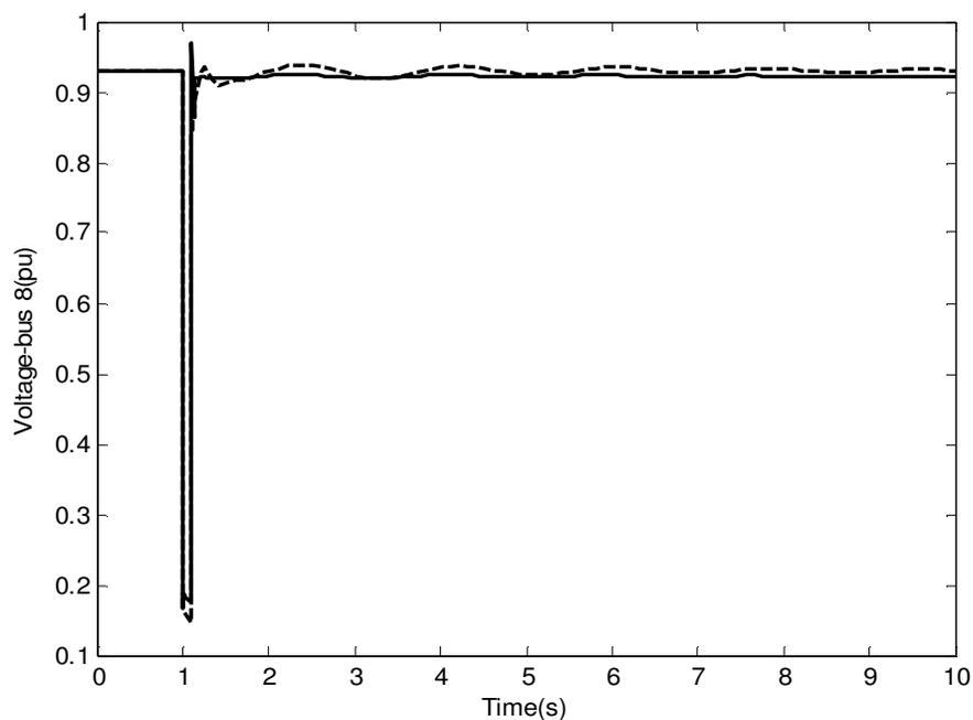
**Figure 8.** Voltage of bus number 8 under scenario 2 in nominal load condition. Solid (with UPFC); Dashed (without UPFC).
