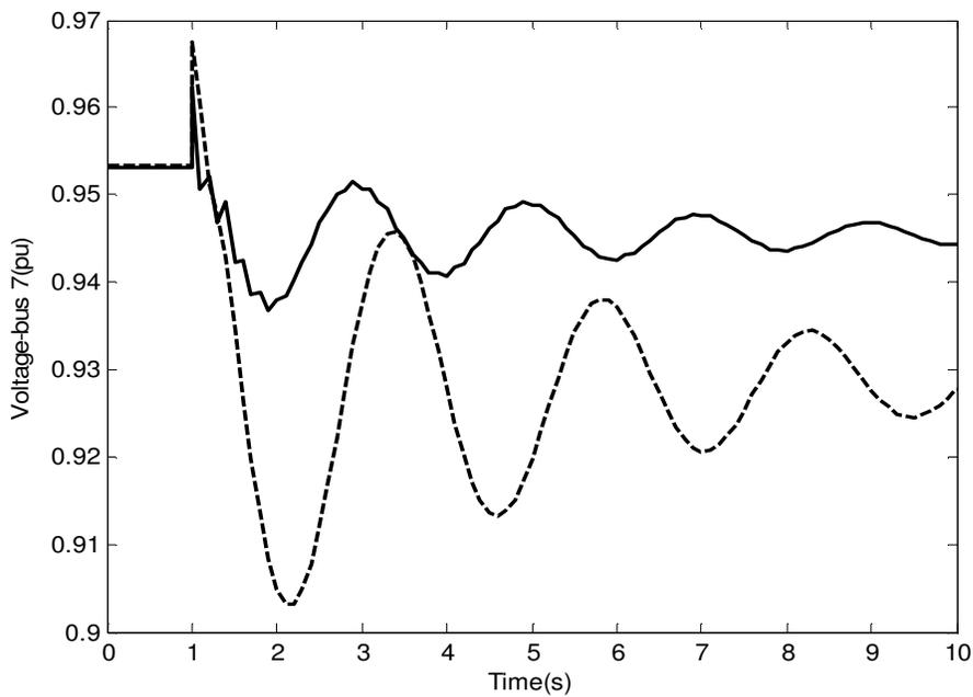
**Figure 5.** Voltage of bus number 7 under scenario 1 in nominal load condition. Solid (with UPFC); Dashed (without UPFC).
