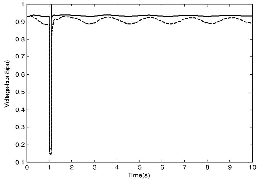
**Figure 10.** Voltage of bus number 8 under scenario 2 in heavy load condition. Solid (with UPFC); Dashed (without UPFC).
