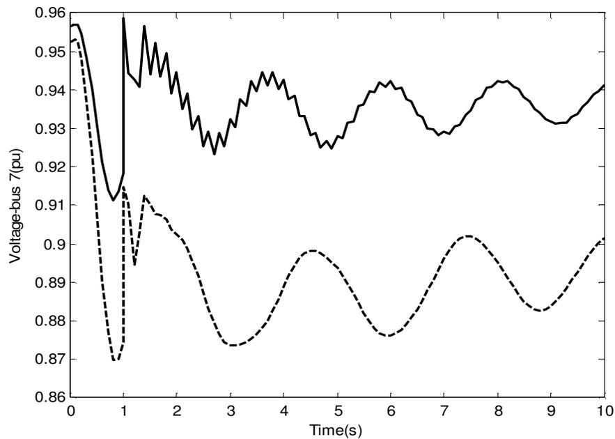
**Figure 7.** Voltage of bus number 7 under scenario 1 in heavy load condition. Solid (with UPFC); Dashed (without UPFC).
