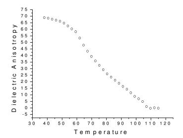
Figure 4. Variation of dielectric anisotropy with temperature.
