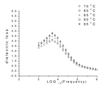
**Figure 2**. Variation of dielectric loss with log<sub>10</sub> (frequency) at different temperatures i.e. 70°, 80°, 85°,90°& 95° C.
