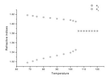
Figure 5. Variation of Refractive indices with temperature.
