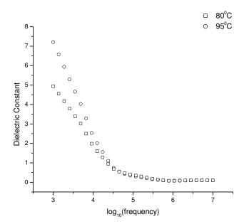
Figure 1. Variation of dielectric constant with log<sub>10</sub> (frequency)
