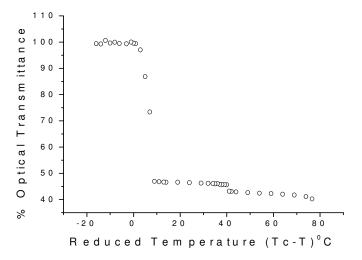
Figure 8. Variation of % Optical Transmittance with reduced temperature
