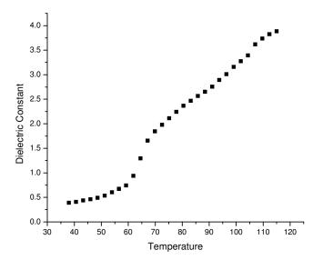
Figure 3. Variation of dielectric constant with temperature.
