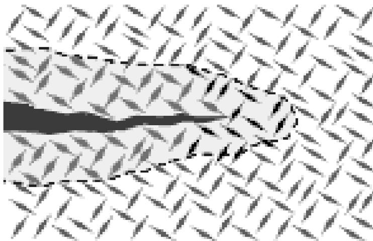
**Figure 8.** Phase transformation at the crack tip.
