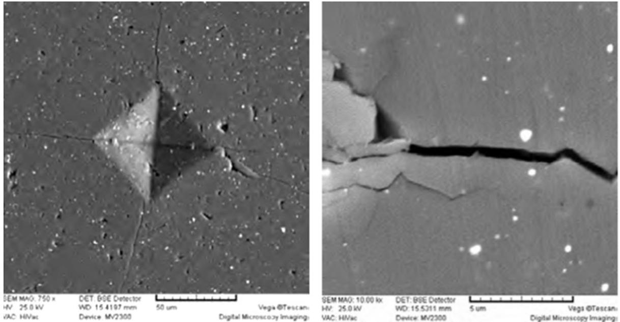
**Figure 9.** SEM photograph of the cracks created by indentation of Vickers pyramid on the raw specimen.
