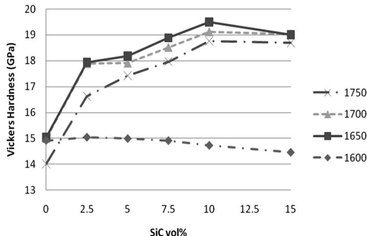
**Figure 3.** Vickers hardness of  $\text{Al}_2\text{O}_3$ -SiC-MgO as a function of sintering temperature and vol% SiC.
