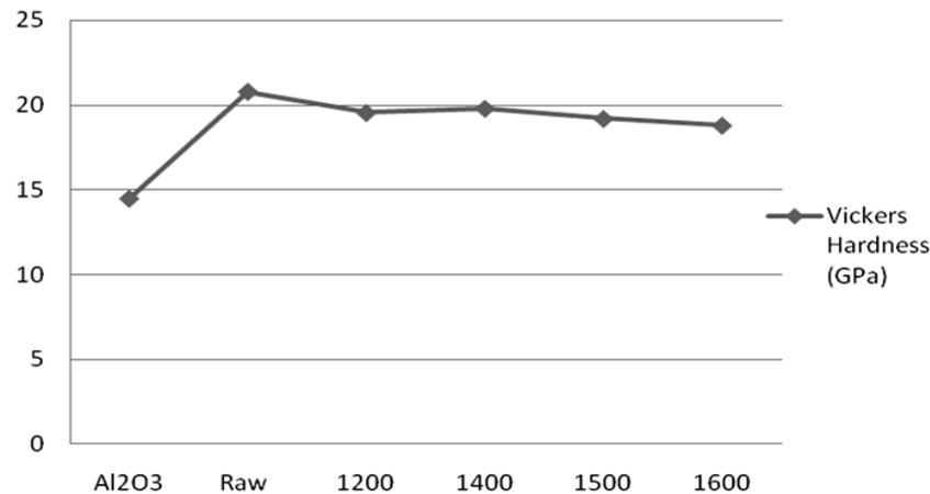
Figure 6. Hardness of the annealed samples.
