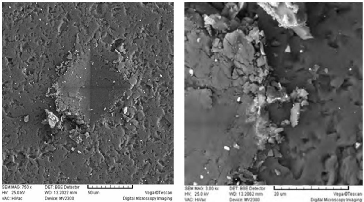
**Figure 10.** SEM photograph of indentation of Vickers pyramid on the 2 h annealed specimen at 1500 °C.
