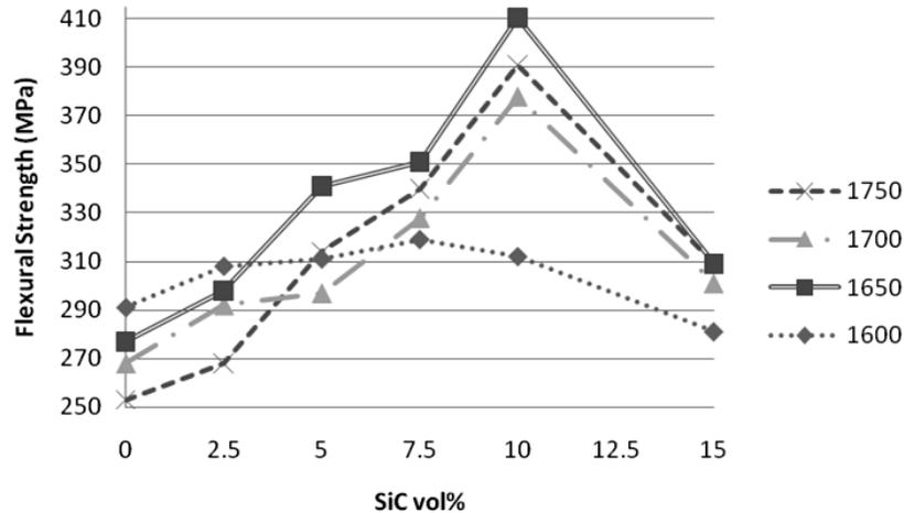
**Figure 1.** Flexural strength of  $\text{Al}_2\text{O}_3\text{-SiC-MgO}$  as a function of sintering temperature and vol% SiC.
