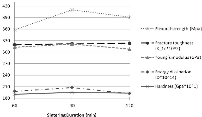
**Figure 4.** Mechanical properties of specimens at different sintering duration at sintering temperature of 1650°C.
