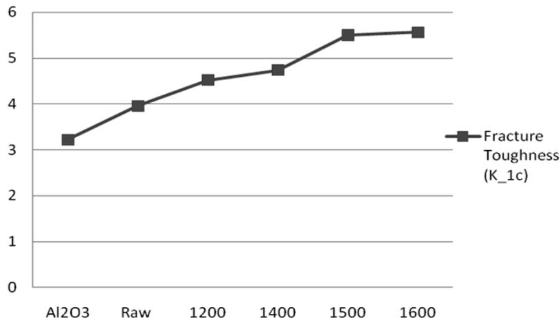
**Figure 7.**  $k_{1c}$  for annealed samples in comparison with pure alumina and raw nanoceramic.
