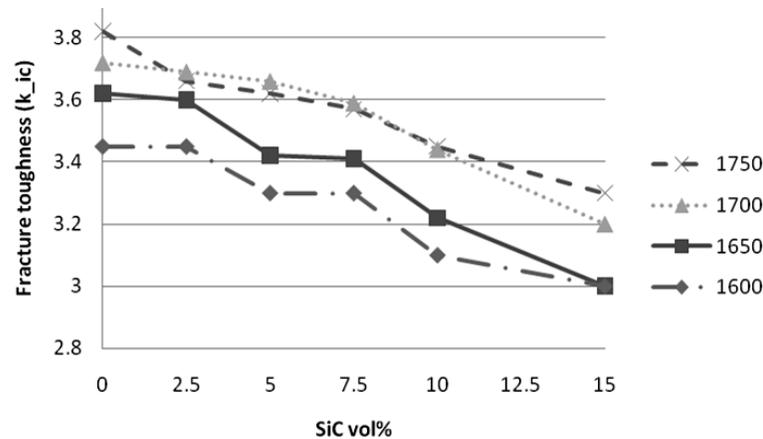
**Figure 2.** Fracture toughness of  $\text{Al}_2\text{O}_3\text{-SiC-MgO}$  function of sintering temperature and vol% SiC.
