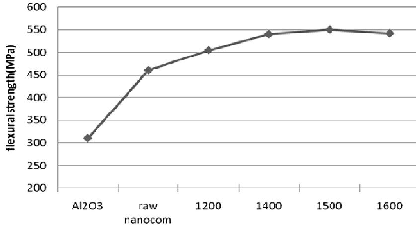
Figure 5. Flexural strength of annealed samples.
