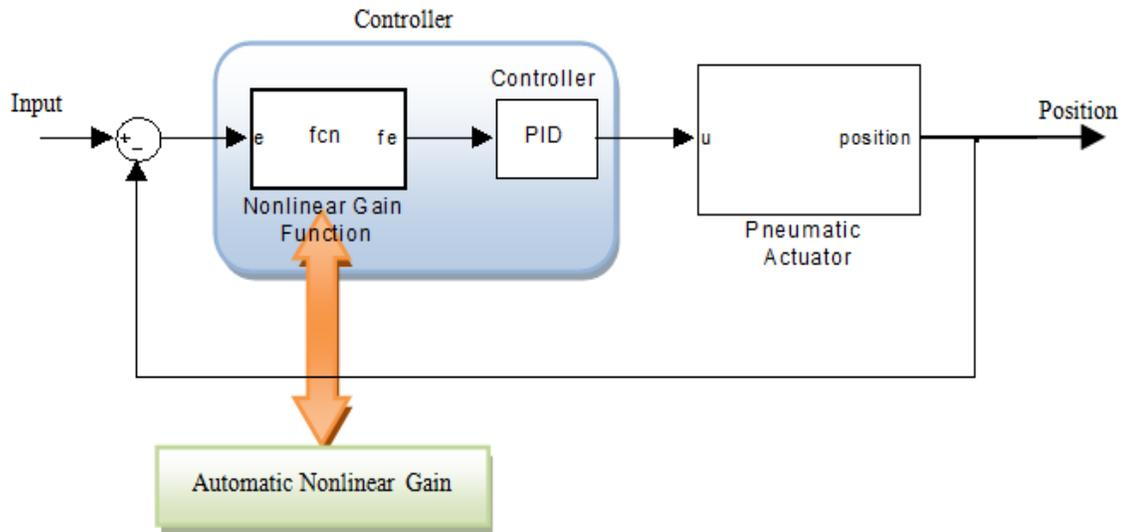
Figure 5. Block diagram of the N-PID control system.
