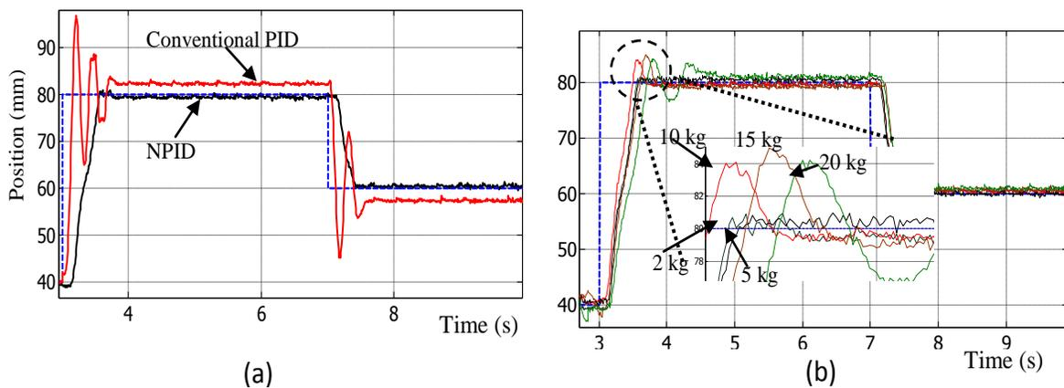
**Figure 16.** Experimental results for the different payload based on step input reference; (a) performance of NPID and conventional PID controller for 2 kg payload (b) NPID controller with payload up to 20 kg.
