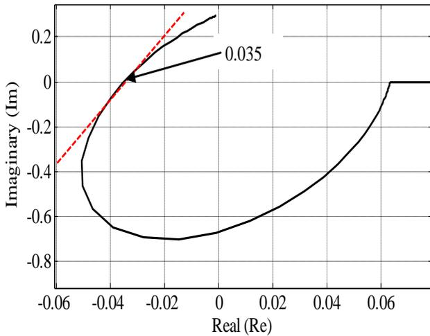
Figure 6. Popov plot of the N-PID control system.
