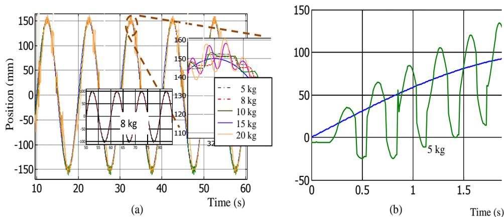
**Figure 18.** Experimental results of payload up to 20 kg based on sinusoidal input reference; (a) NPID controller can well accommodate a payload up to 20 kg, (b) conventional PID controller cannot sustain when the payload increase more than 5 kg.
