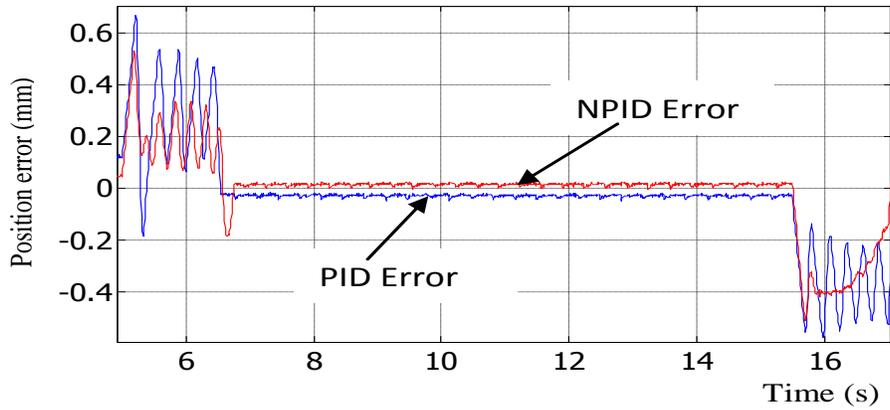
**Figure 14.** Experimental result of position error signal based on trapezoidal reference signal.
