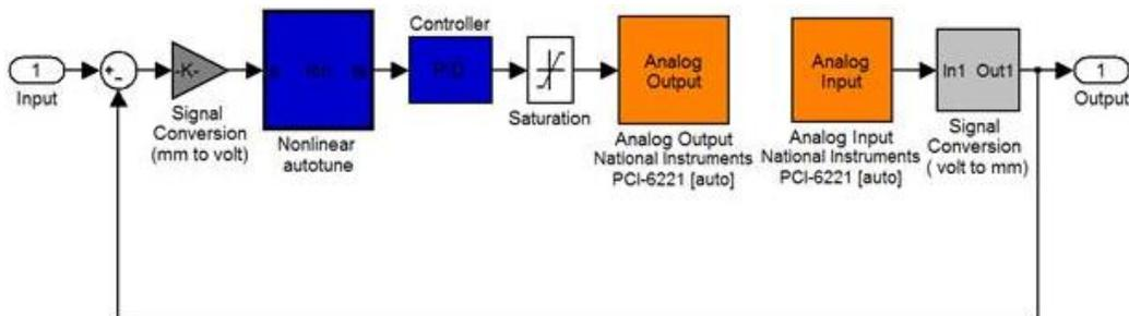
Figure 10. Implementation block diagram of the real system.
