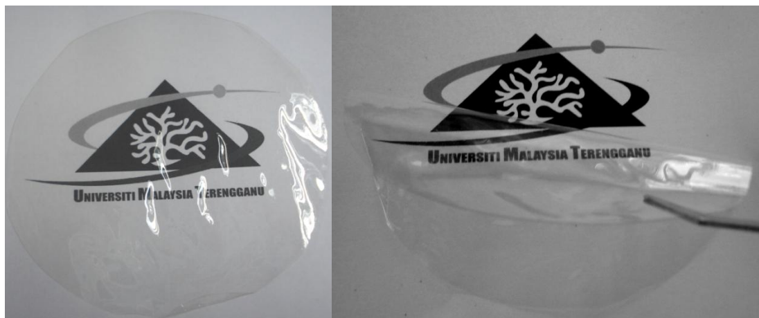
Figure 1. The highly translucent and flexible CMC-AN solid polymer electrolyte films.
