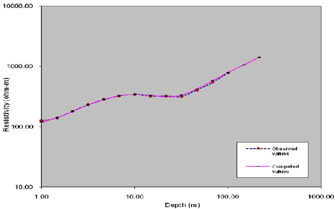
Figure 2. Field data, theoretical curve and the layer model of wire Road, Obiaruku.
