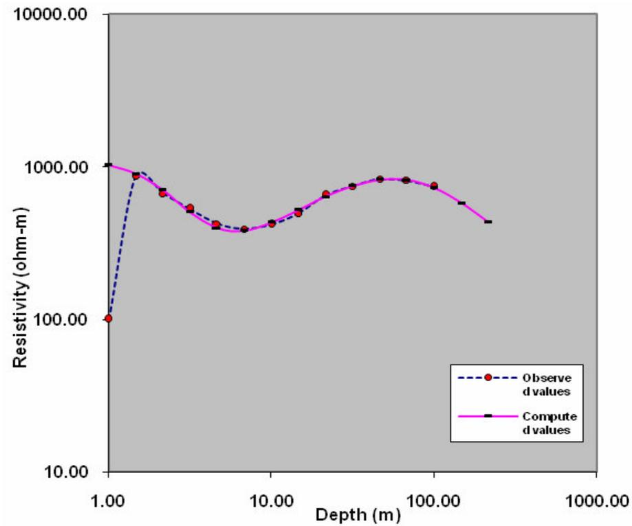
Figure 5. Field Data, theoretical curve and the layer model of Adonishaka in Ebedei, Adonishaka Ebedei, showing observed (field) and theoretical resistivity data curves; and interpreted layer parameters.
