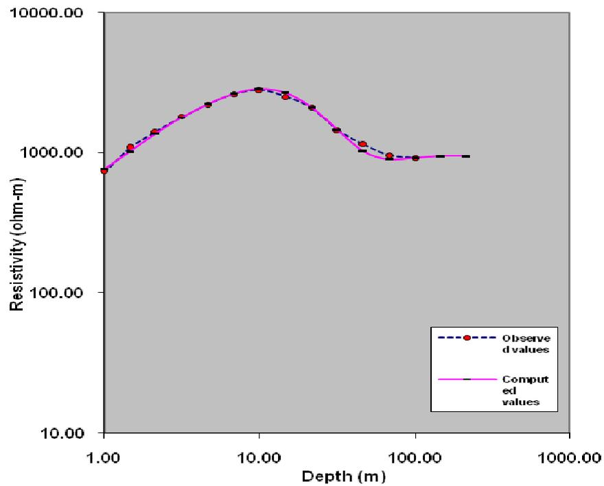
Figure 4. Field data, theoretical curve and the layer model of Umukwata off New Sapele/Agbor road.
