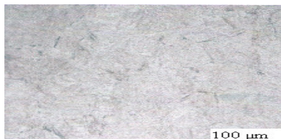
Figure 2(i). The microstructure of furnace cooled AISI 1040 steels.
