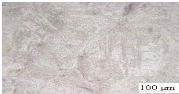
Figure 2(g). The microstructure of water quenched AISI 1060.
