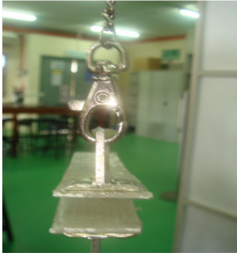
Figure 10. Crack opening displacement ( \delta ) is extended when load is applied.
