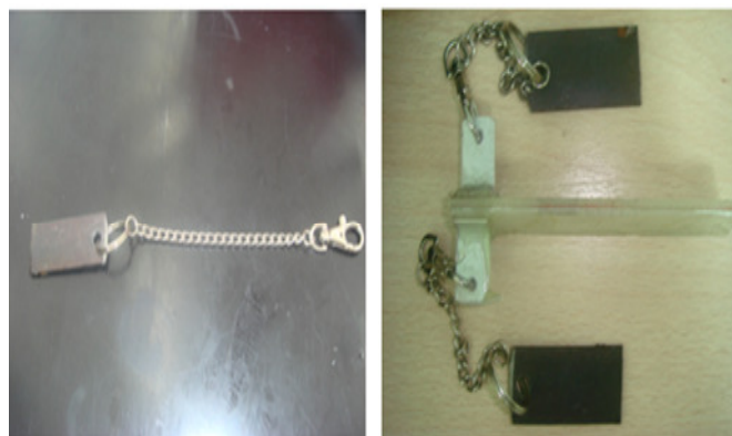
Figure 7. Chains hinged to loading blocks.
