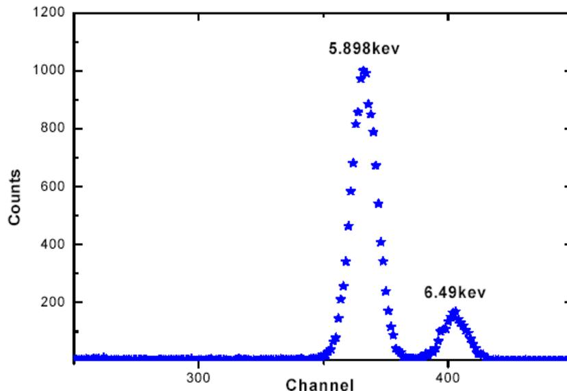
Figure 4. <sup>55</sup>Fe spectrum without absorber.
