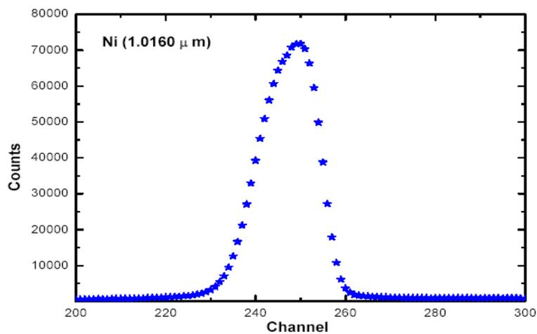
Figure 8. Transmitted alpha spectrum through Nickel target.
