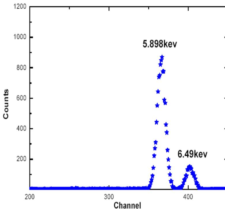
Figure 5. <sup>55</sup>Fe spectrum with aluminium absorber.
