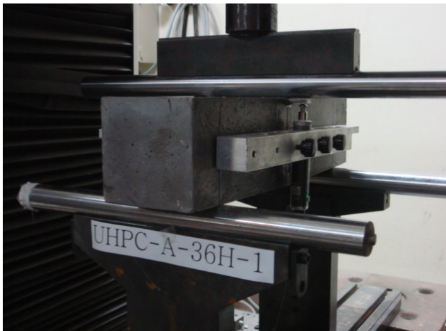
Figure 2. Overall view of three-point bending test setup.
