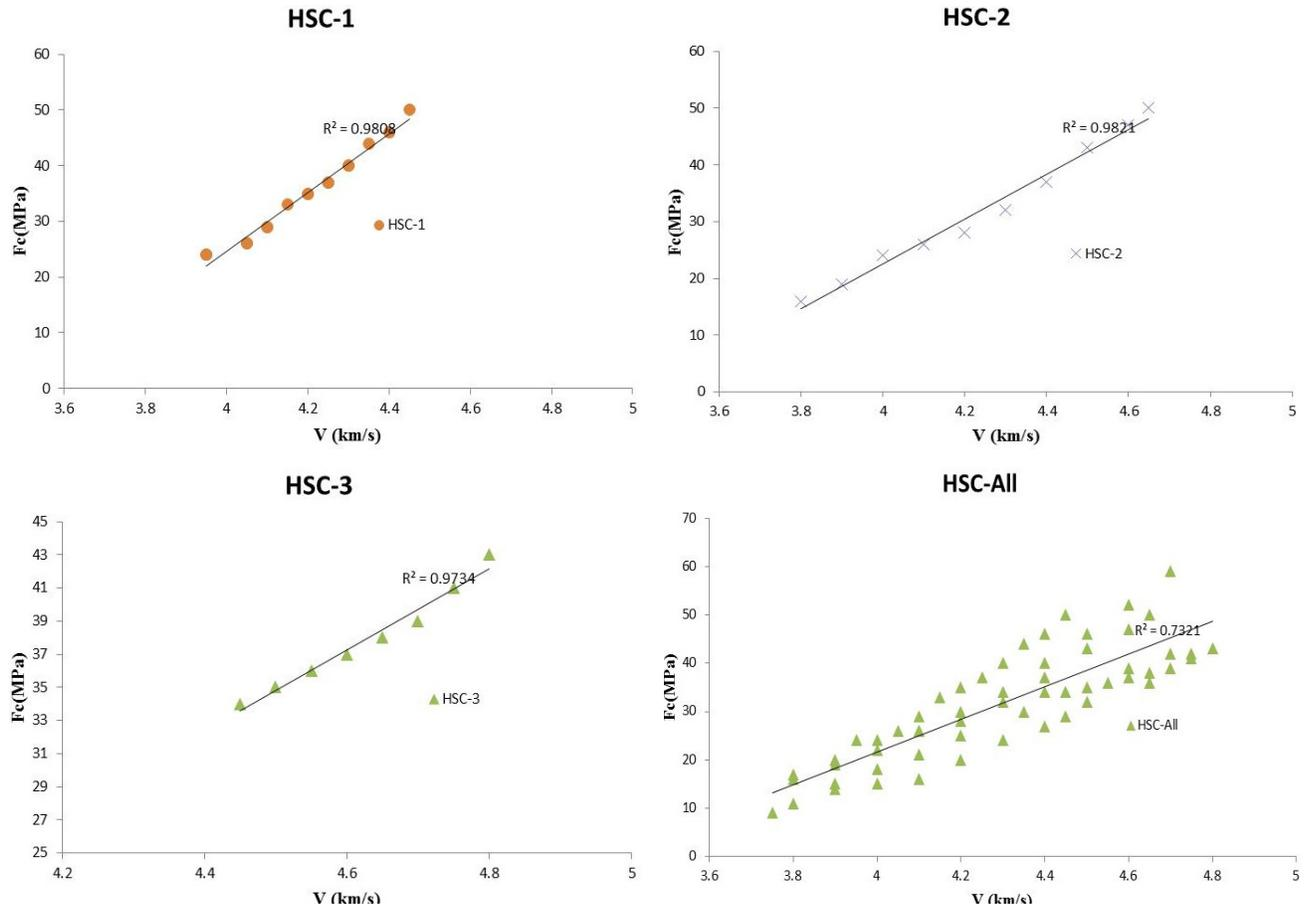
**Figure 8.** The effect of choosing selected concrete mix and all concrete mix on UPV.
