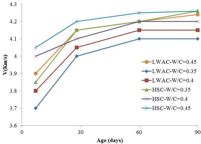
Figure 5. The effect of cement content on UPV.
