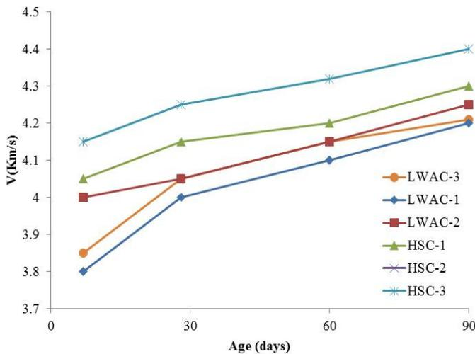
Figure 4. The effect of age on UPV rates for HSC and LWAC.
