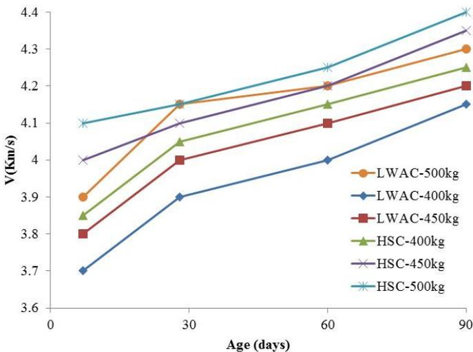
Figure 6. The effect water cement ratio on UPV.
