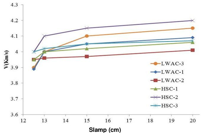
Figure 7. The effect of concrete slump on UPV (for slump less and more than 12 cm).
