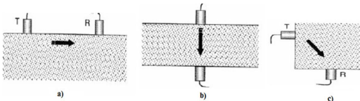
Figure 2. The arrangement of probe of pulse velocity measurement: Direct (a), semi-direct (b) indirect (surface) transmission
