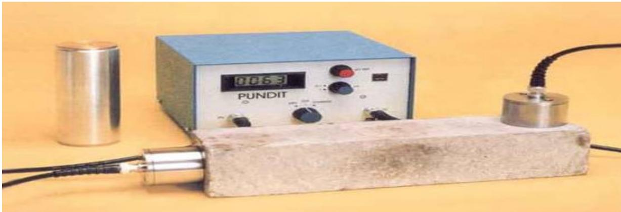
Figure 1. Pulse velocity testing equipment (PUNDIT).
