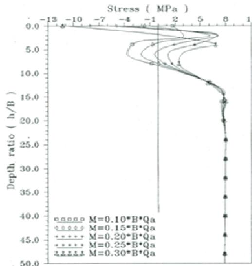
**Figure 9.** Effect of moment loading on the stress distribution along the shaft of driven pile in sand.
