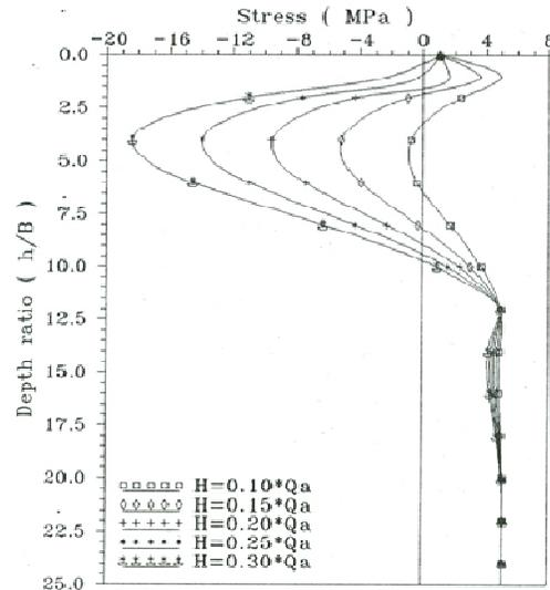
**Figure 4.** Effect of lateral loading on the stress distribution along the shaft of bored pile in sand.
