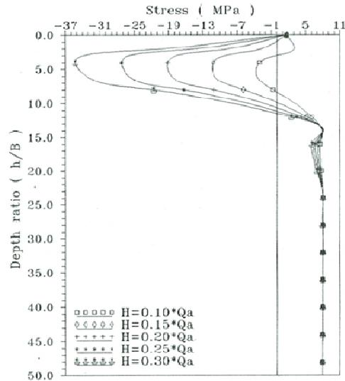
**Figure 10.** Effect of lateral loading on the stress distribution along the shaft of driven pile in sand.
