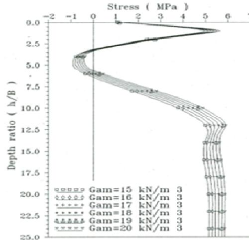
**Figure 8.** Effect of unit weight of soil on the stress distribution along the shaft of bored pile in sand.
