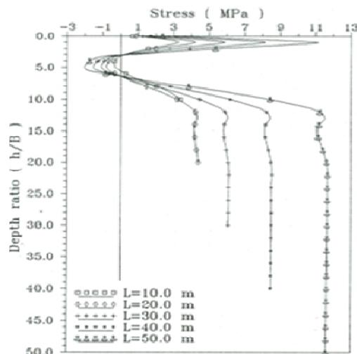
**Figure 5.** Effect of pile length on the stress distribution along the shaft of bored pile in sand.
