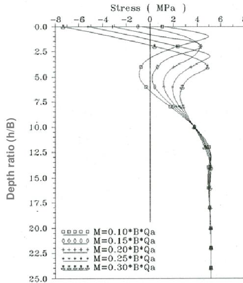
Figure 3. Effect of moment loading on the stress distribution along the shaft of bored pile in sand.
