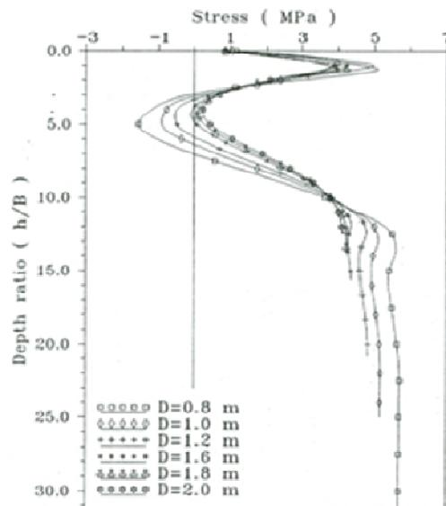
**Figure 6.** Effect of diameter on the stress distribution along the shaft of bored pile in sand.
