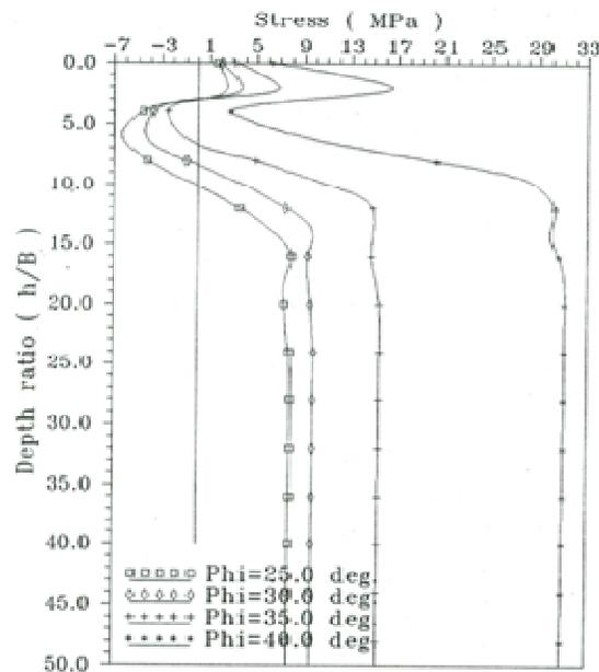
**Figure 13.** Effect of friction angle on the stress distribution along the shaft of driven pile in sand.
