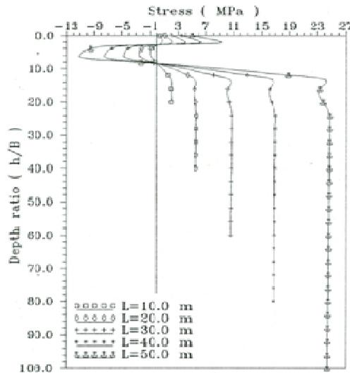
**Figure 11.** Effect of pile length on the stress distribution along the shaft of driven pile in sand.
