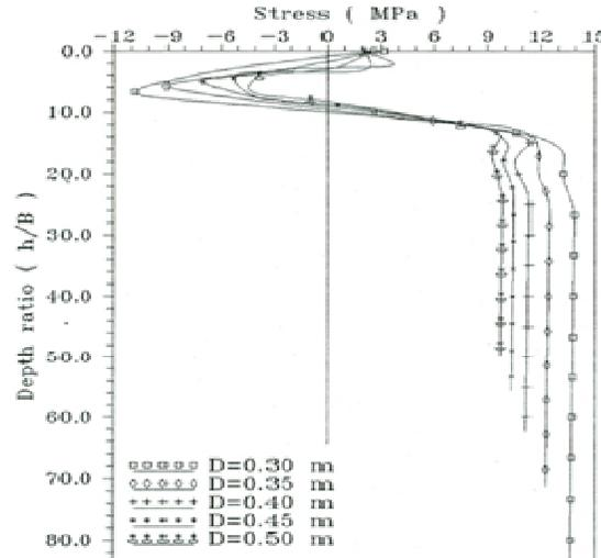
**Figure 12.** Effect of diameter on the stress distribution along the shaft of driven pile in sand.
