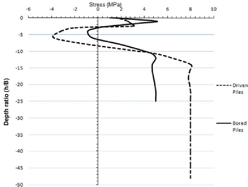
Figure 2. Stress distribution for driven and bored pile embedded in sand.
