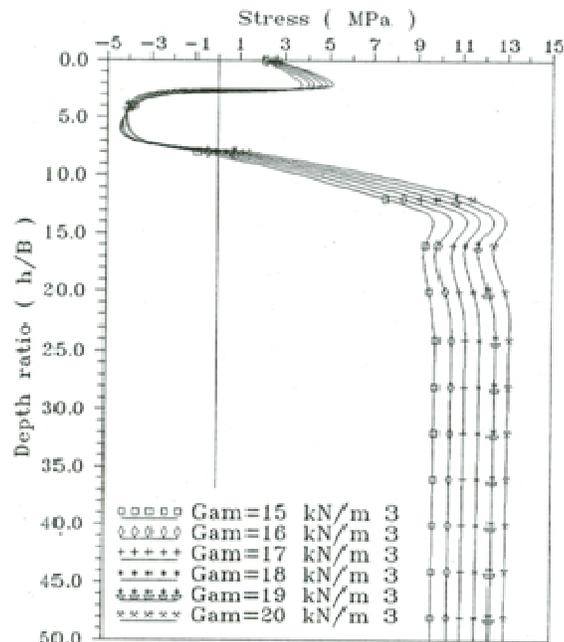
**Figure 14.** Effect of unit weight of soil on the stress distribution along the shaft of driven pile in sand.
