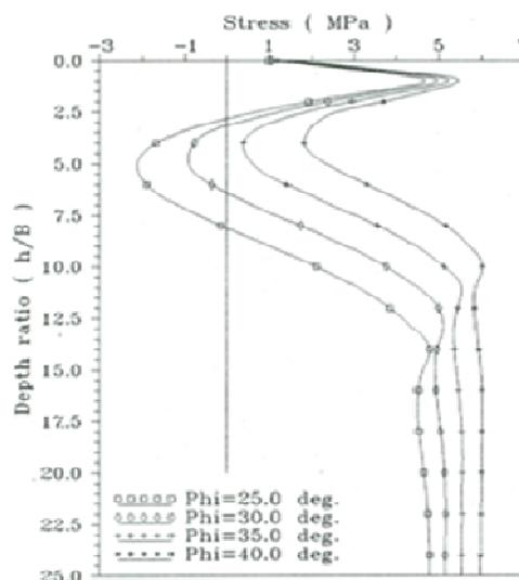
**Figure 7.** Effect of friction angle on the stress distribution along the shaft of bored pile in sand.
