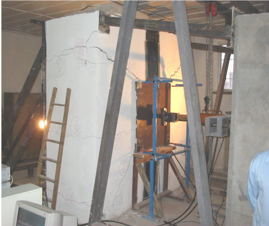
Figure 19. Loading and final surface cracking of test specimen S_{(FRP)} with the FRP strip applied at mid-centre.
