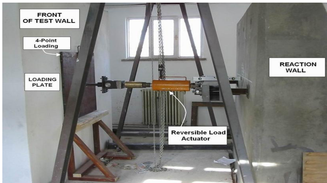
Figure 10. The reversible loading set-up.
