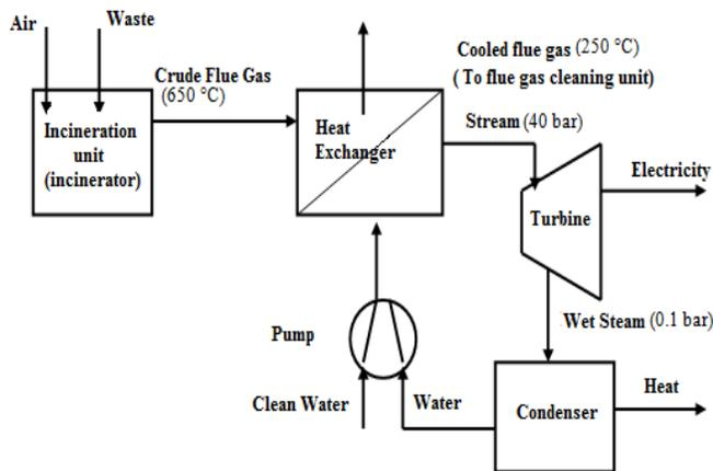
Figure 2. Schematic diagram of electricity generation.
