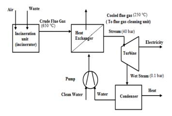
Figure 2. Schematic diyagram of electricity generation.
