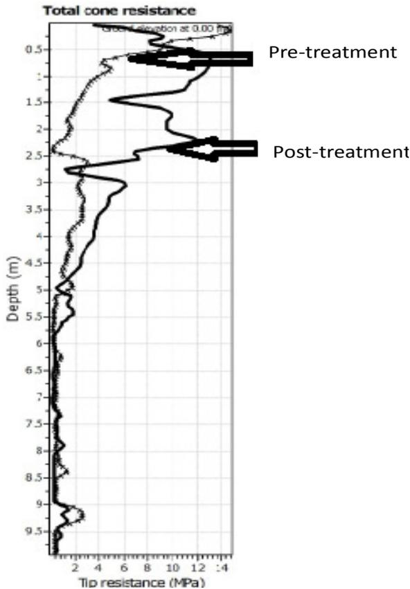
**Figure 2.** Overlay drawing of pre-treatment and post-treatment cone resistance at project site.
