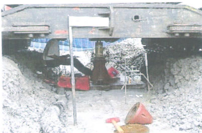
**Figure 3.** Plate bearing test.
