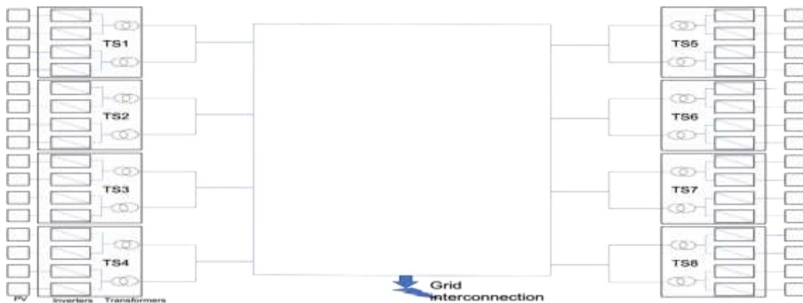
**Figure 1.** Simplified diagram of Diass solar PV plan.**Table 3.** Technical characteristics of PV system in STC.
