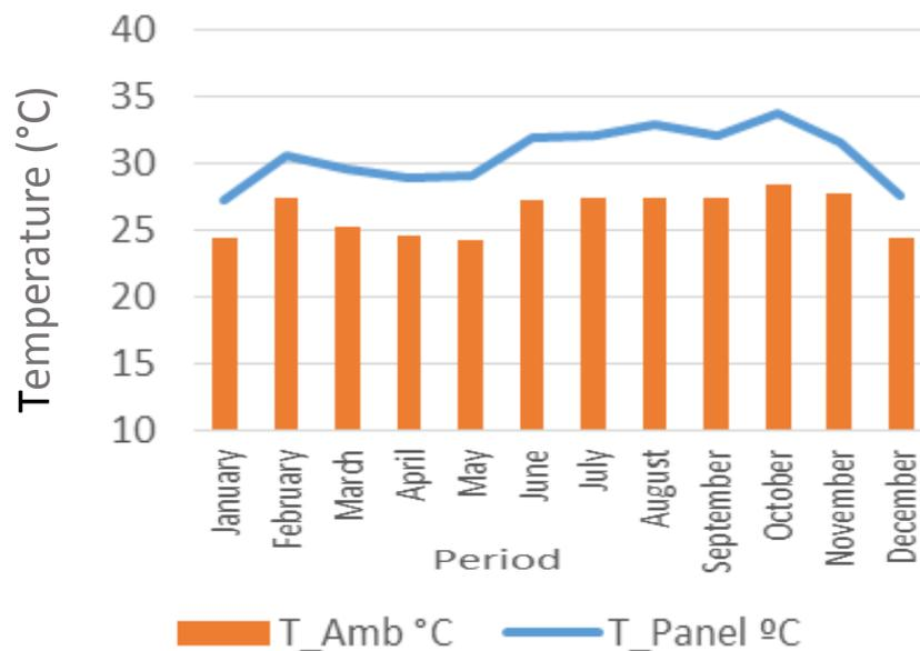
**Figure 3.** Monthly variation of daily average module temperature and ambient temperature.
