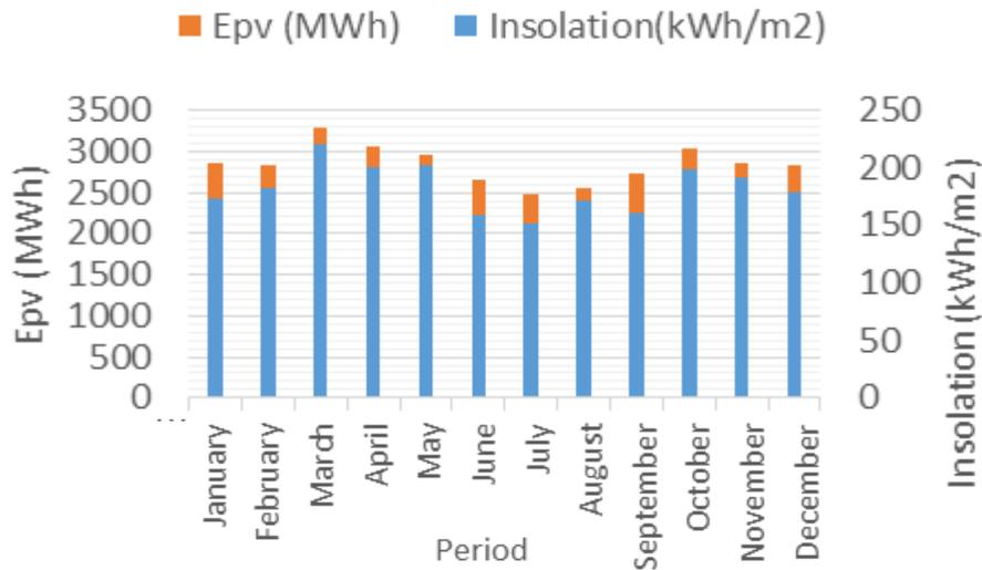
**Figure 4.** Monthly variation of daily average insolation and the monthly total energy output from PV modules.
