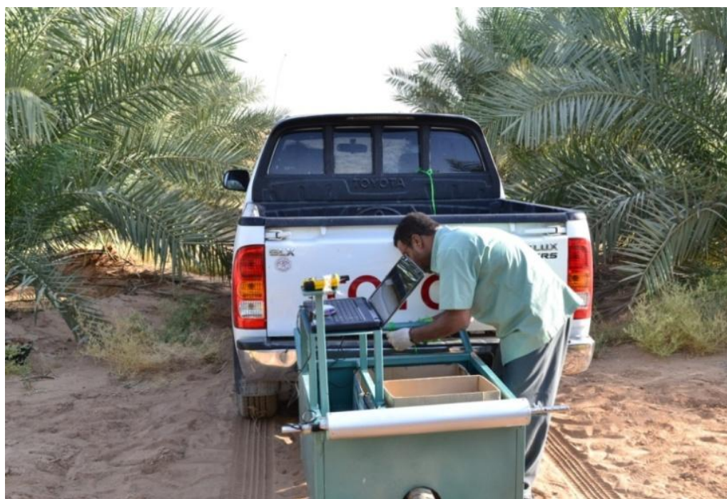
Figure 2. The mole detector, GPS and laptop are placed on a fabricated carriage and pulled by a vehicle over the field.
