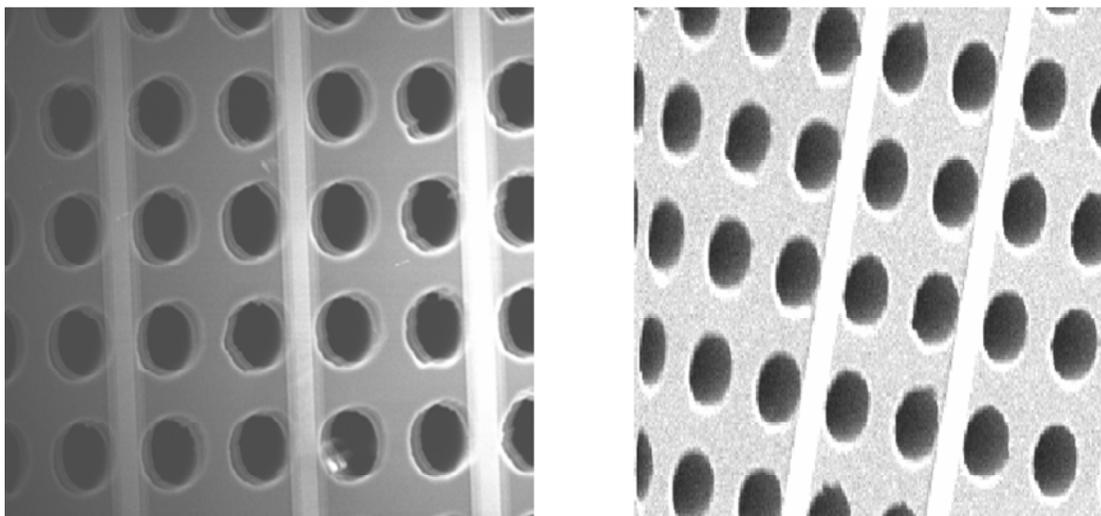
**Figure 1.** Dependence of SE yields on the angle of tilt (right) relative to the primary-electron beam (zero angles correspond to perpendicular incidence (left)). Data points represent experimental measurements for chip.
