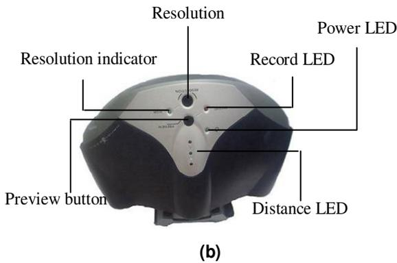
Figure 1. Handyscan 3D laser scanner. (a) main view; (b) Top view.
