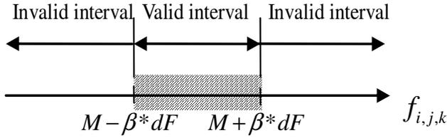
Figure 5. The elimination interval schematic of quartile method.
