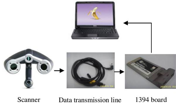
Figure 2. System components.
