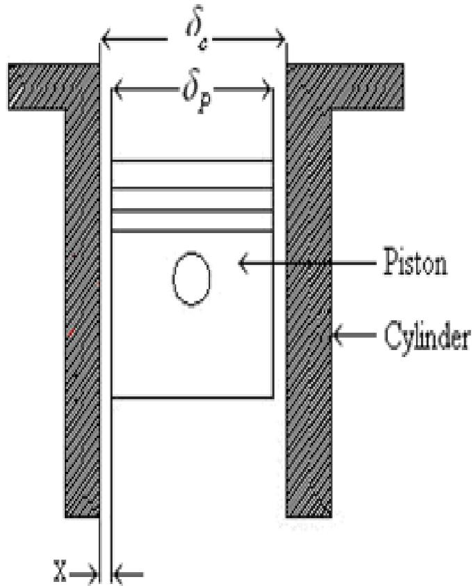
Figure 1. Piston and cylinder assembly.
