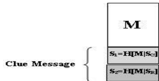
Figure 7. Clue message structure where 1st Hashed value and 2nd Hashed value are broadcasted along with the message M .
