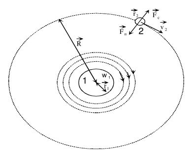
**Figure 1.** Two-dimensional model of gravitational interaction of two bodies. The forces are shown acting on body 2:  $F_c$ : The centrifugal force;  $F_n$ : The force of attraction of body 2 from body 1;  $v_2$ : Linear velocity of body 2 at the orbit; R: The radius of the orbit;  $F_n$ : The radius of body 1;  $F_n$ : The radius of body 1;  $F_n$ : The radius of body 1;  $F_n$ : The radius of body 1.
