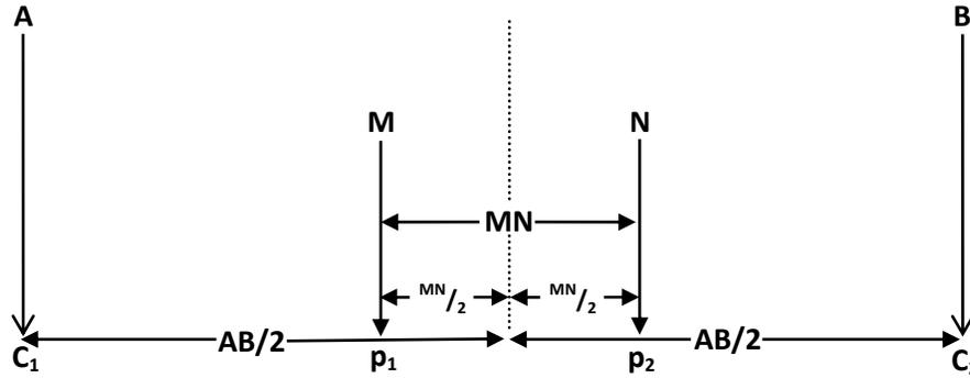
**Figure 6.** Schlumberger electrode configuration.
