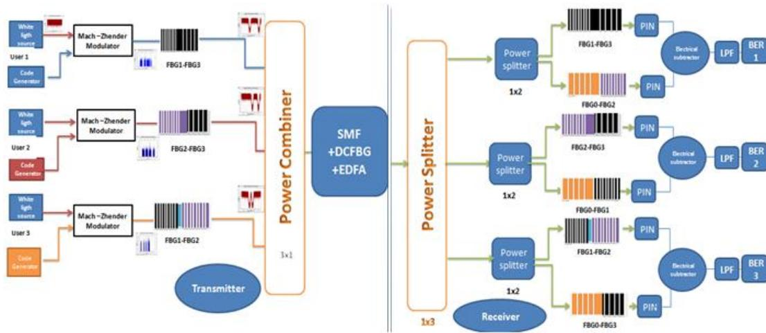
Figure 2. Block diagram of 3 user Incoherent SAE-OCDMA.
