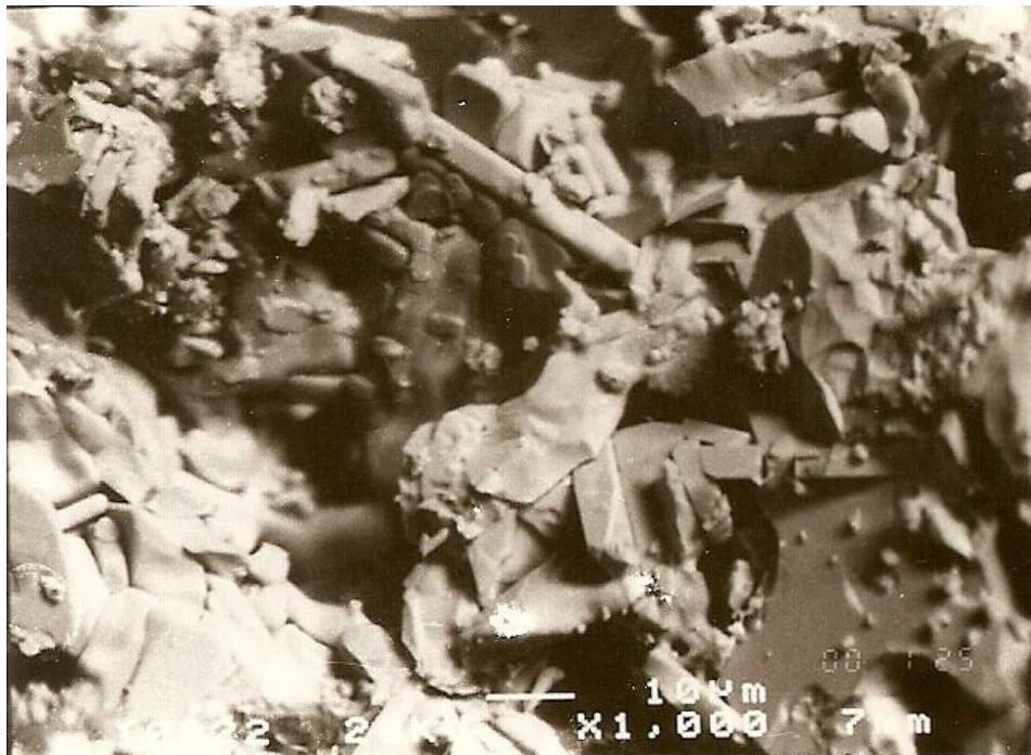
Figure 14. Morphology of fracture surface of compound \text{Bi}_2\text{Sr}_2\text{Ca}_{n-1}\text{Cu}_n\text{O}_{2n+46} , n, 4.5 + \text{Pb} .
