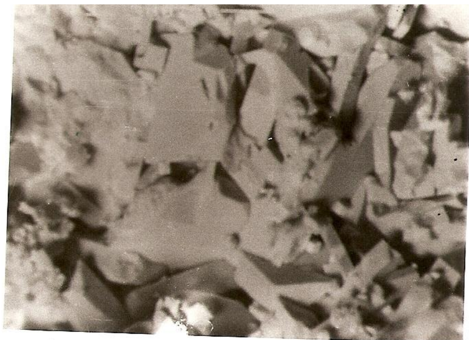
Figure 11. Morphology of fracture surface of compound \text{Bi}_2\text{Sr}_2\text{Ca}_{n-1}\text{Cu}_n\text{O}_{2n+4\delta} . n , 3 + Pb.
