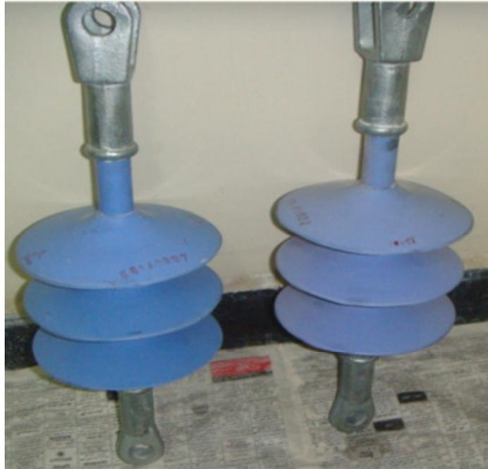
**Figure 2a.** Photograph of tested insulator.
