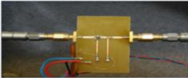
Figure 18. Implemented circuit for single stage LNA.
