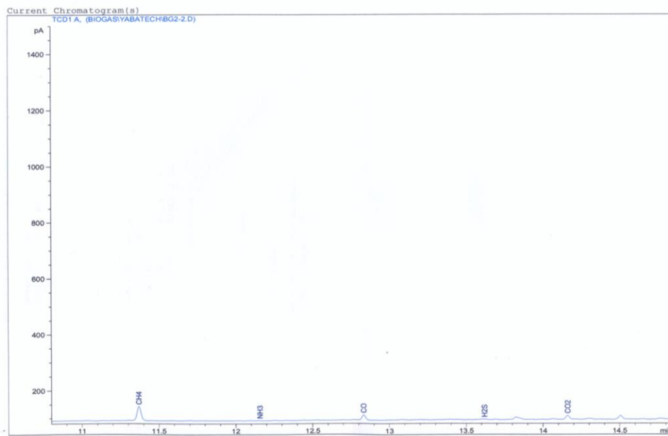
Figure 7. The variation of peaks of component hydrocarbons and other gases processed with the waste (Treatment E: Corncob, rice chaff, goat dung (75%) and dog dung (25%)).
