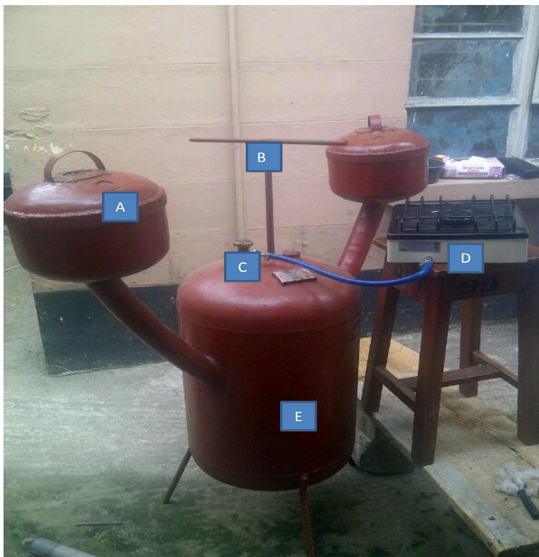
Figure 1. Picture of the bioreactor. A- Feeder point, B- Stirrer, C- Nozzle for gas outlet, D- Gas cooker and E- Digester tank.
