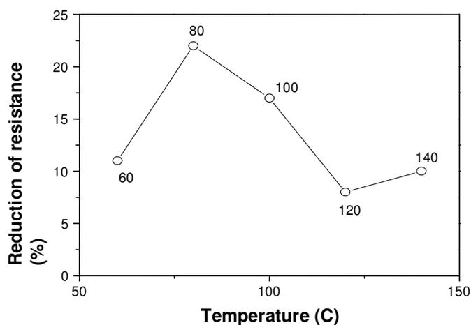
**Figure 4.** Influence of substrate temperature during hydrogenation process on reduction of resistance.
