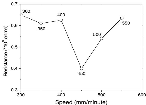
Figure 2. The electrical resistance versus dipping speeds.
