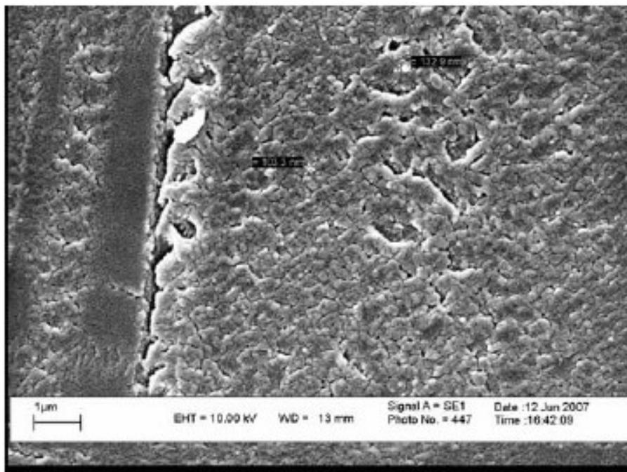
**Figure 8.** SEM micrograph after hydrogenation.
