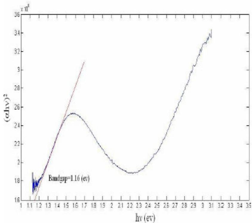
**Figure 3.** Optical bandgap of the PEDT/PSS film.
