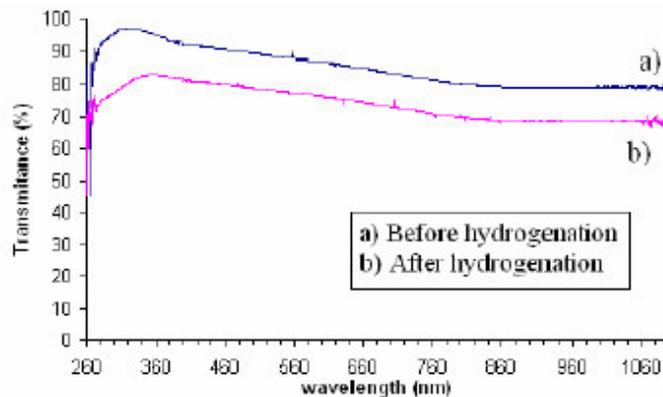
**Figure 6.** Optical transmission spectra of the PEDT/PSS film before and after hydrogenation.
