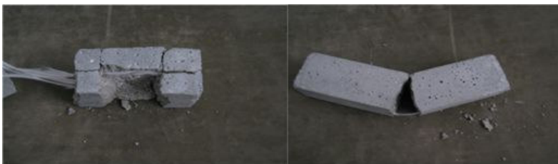
Figure 16. Specimen 0-L-0 and C-0-L having undergone a compression.
