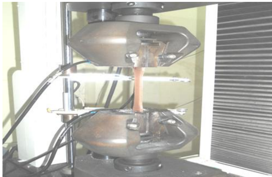
Figure 3. Tensile strength testing of specimen.
