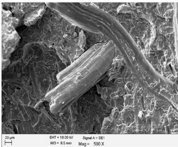
Figure 8. SEM image of Impact fractured surfaces of HYBRID PP composite.
