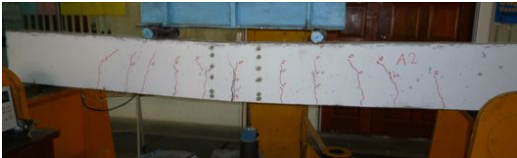
Plate 1. Failure mode of beam A1.
