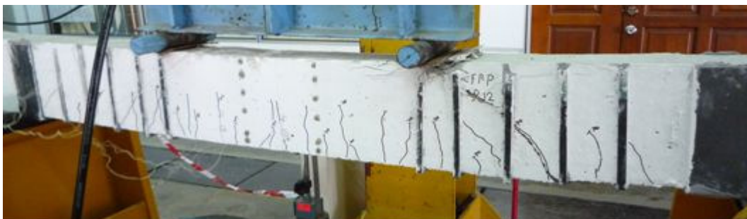
Plate 3. Failure mode of beam B2.
