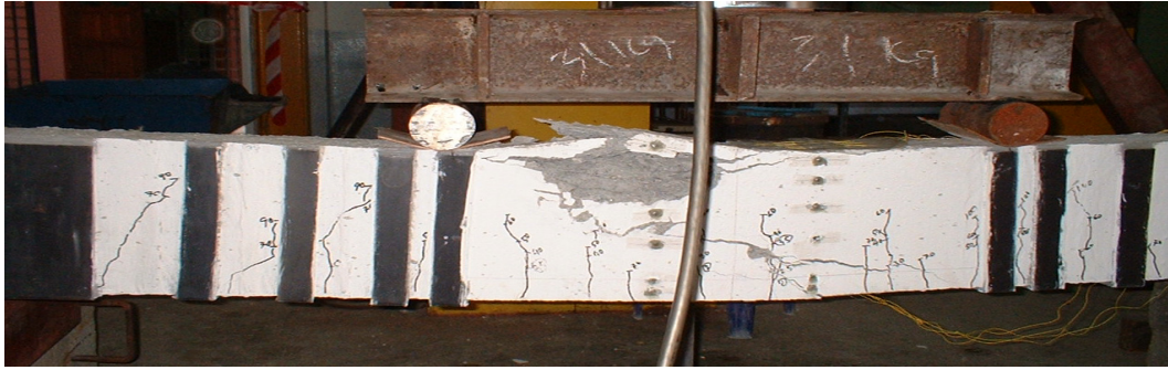
Plate 4. Failure mode of beam B3.
