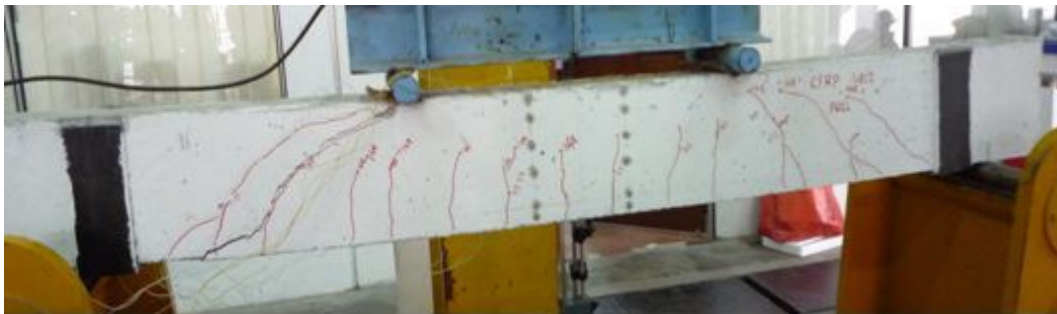
Plate 2. Failure mode of beam B1.
