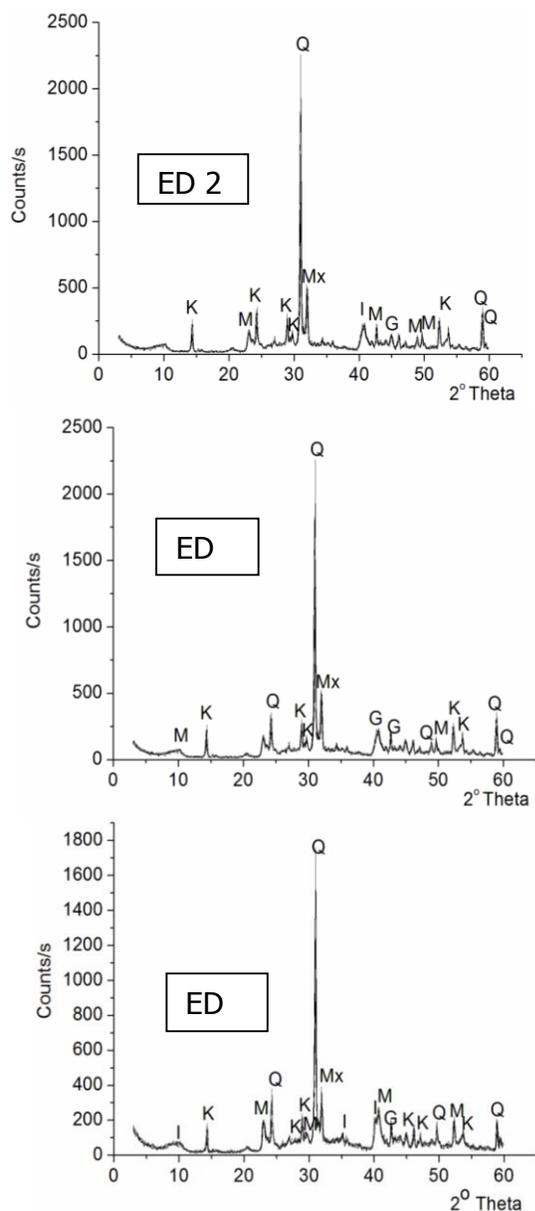
**Figure 4.** X-ray diffractogram of representative samples from Ediki kaolin occurrence (K, kaolinite; M, muscovite; Q, quartz; I, illite; G, goethite; Mx, microcline).
