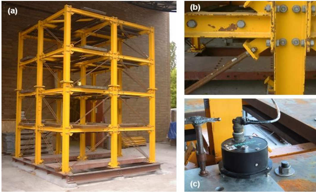
Figure 1. (a) Benchmark structure, (b) beam-column connection and (c) a sample accelerometer.
