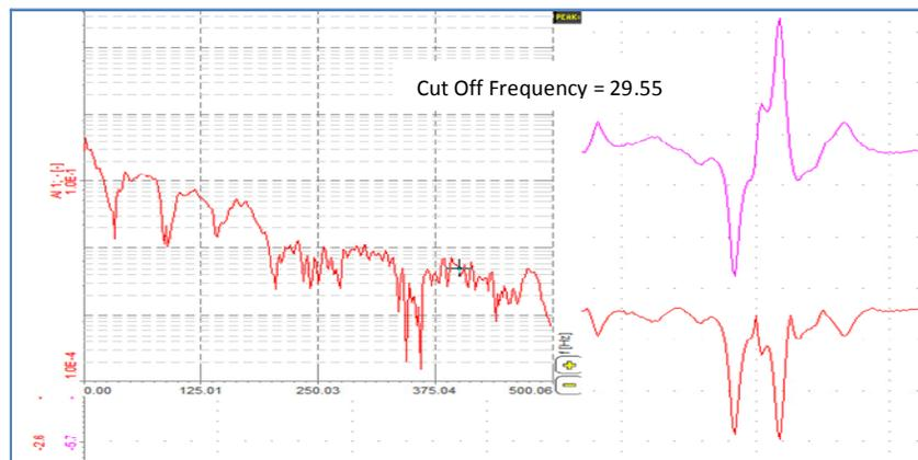
**Figure 27.** Rectified voltage on time and frequency domain for length of 300 mm, which occurred at cut off frequency of 29.55 Hz.
