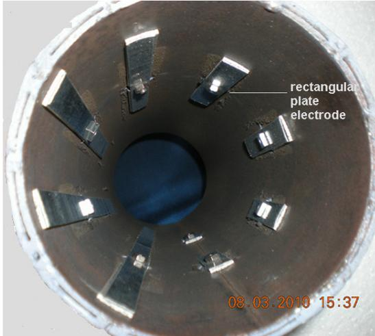
**Figure 3.** Rectangular plate electrodes mounted inside the pipe.
