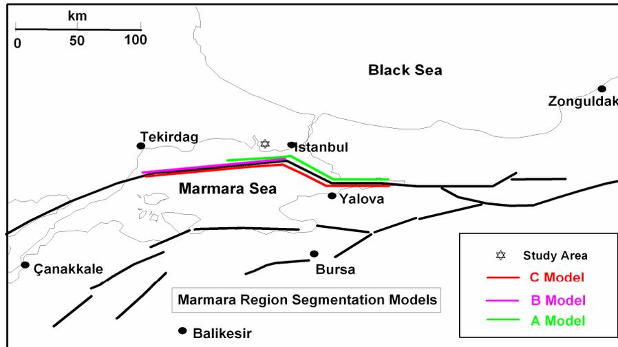
**Figure 1.** For Marmara region, it was assumed four models (A, B and C) for seismic hazard. Model A: approximately 119 km rapture length; Model B: approximately 108 km rapture length; Model C: approximately 174 km rapture length (map is redrawn form JICA-IBB Report, 2002).
