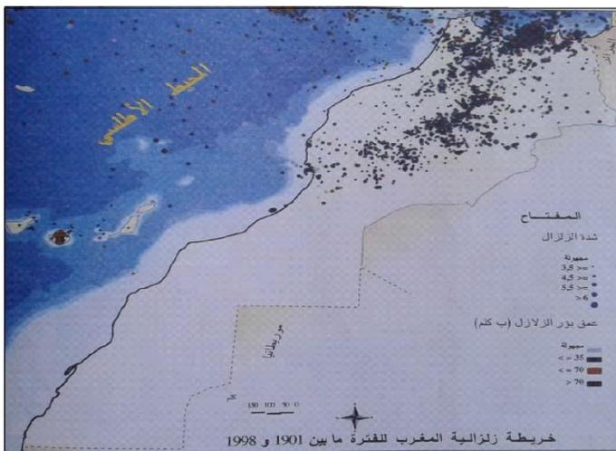
Picture 7. Map of seismic zones in Morocco done by the Ministry of Housing from 1990 referring to scientific institute data (p 23).
