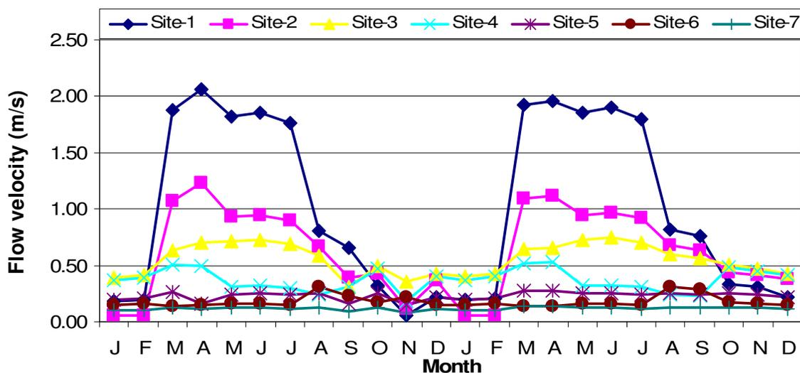
**Figure 2.** Temporal variations of flow velocity ( $\text{m S}^{-1}$ ) at different study sites during study period of January 2005 to December 2006.
