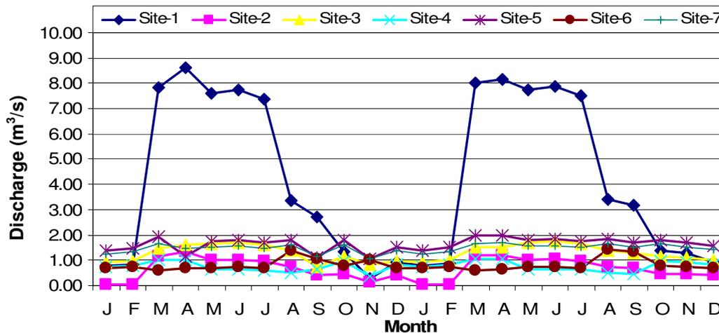
**Figure 3.** Temporal variations of discharge ( $\text{m}^3 \text{S}^{-1}$ ) at different study sites during study period of January 2005 to December 2006.**Table 3.** Doodhganga drainage basin and stream channel geomorphological characteristics.
