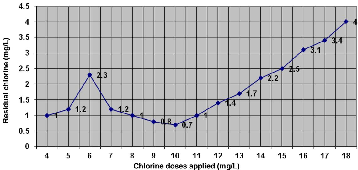
**Figure 4.** Chlorine residuals versus chlorine dose (Single breakpoint when ammonia is  $>0.4$  mg/L and nitrate  $<0.1$  mg/L).
