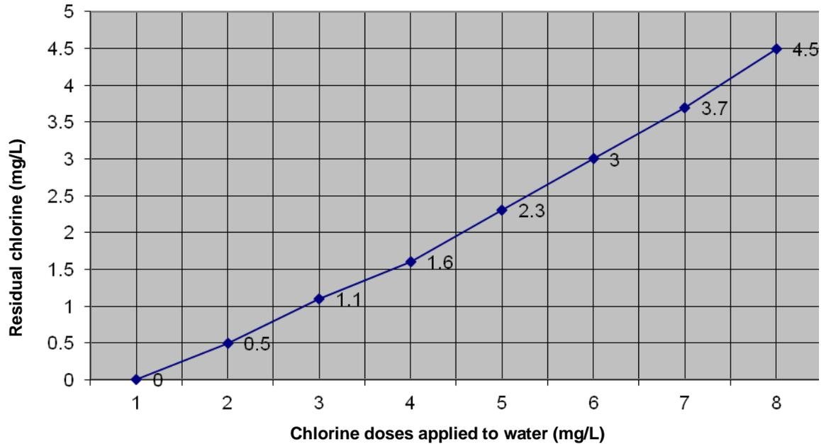
**Figure 3.** Chlorine residuals versus chlorine dose (No breakpoints when ammonia is  $<0.4$  mg/L and nitrate  $>0.1$  mg/L).
