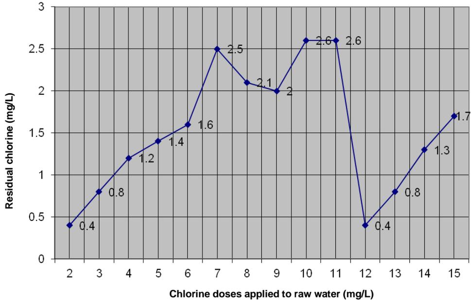
**Figure 1.** Chlorine residuals versus chlorine dose (Double breakpoints when ammonia is  $>0.4$  mg/L and nitrate  $>0.1$  mg/L).
