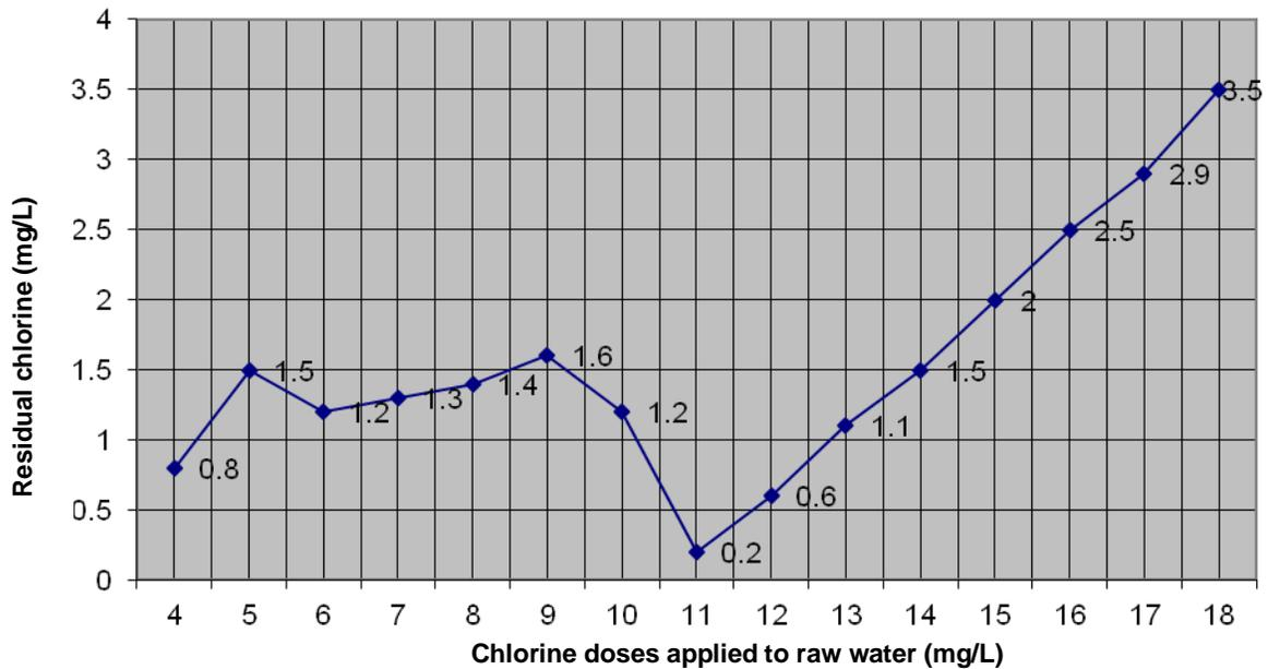
**Figure 2.** Chlorine residuals versus chlorine dose (Double breakpoints when ammonia is  $>0.4$  mg/L and nitrate  $>0.1$  mg/L).
