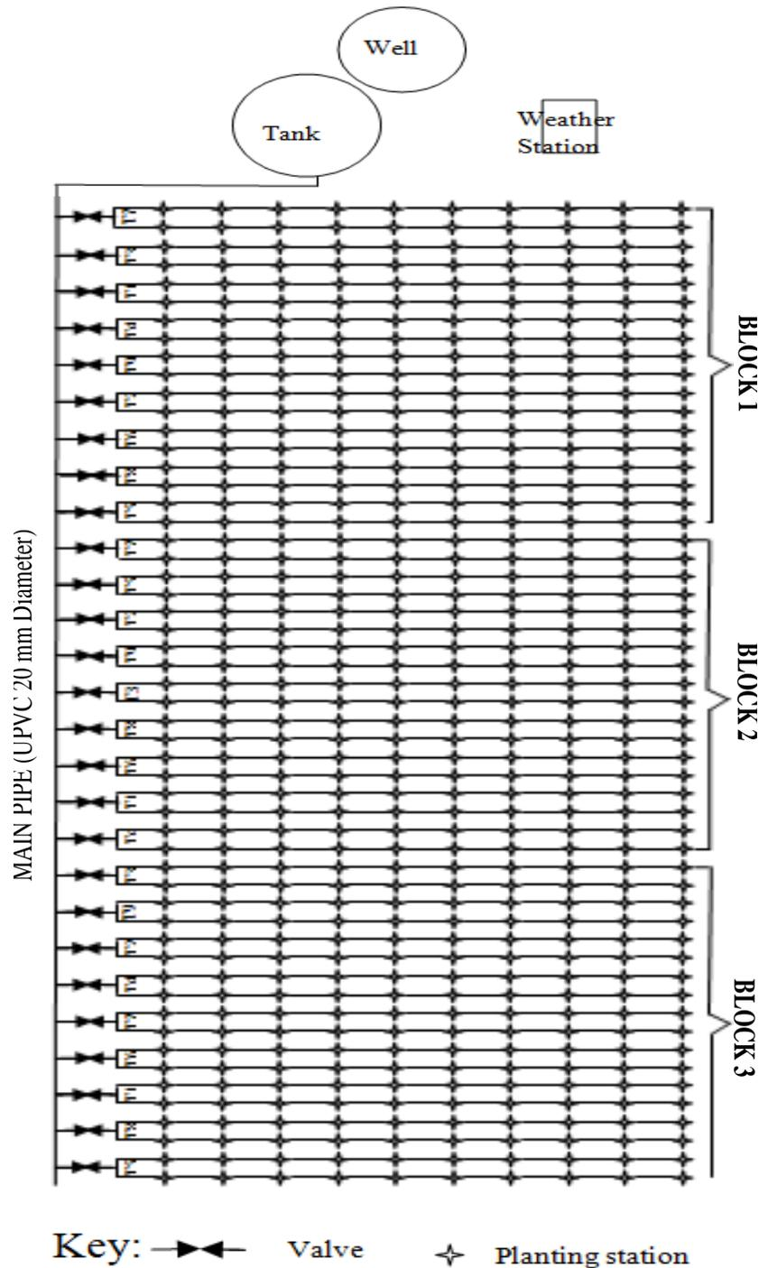
Figure 2. Irrigation layout.
