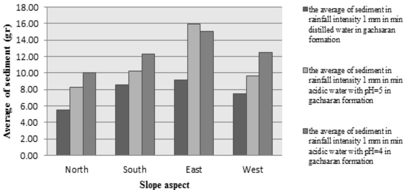
**Figure 2.** The average of sediment with rainfall intensity 1 mm/min in precipitation various density in Gachsaran Gypsum Formation.
