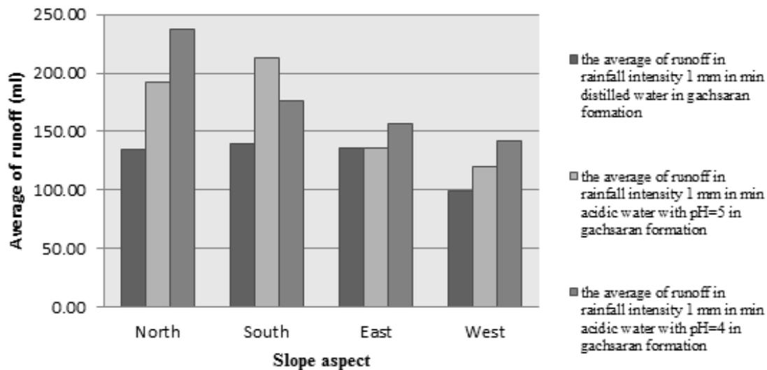
**Figure 3.** The average of runoff with rainfall intensity 1 mm/min in precipitation various density in Gachsaran Gypsum Formation.
