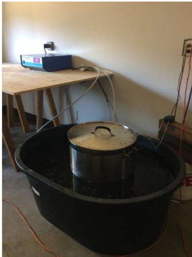
Figure 1. Ultrasonic setup at Elkins Distilling Co. Shows wave generator, immersion bath with ultrasonic transducer, and stainless-steel reaction vessel containing whisky, wood chips, and air pump. Source: Author
