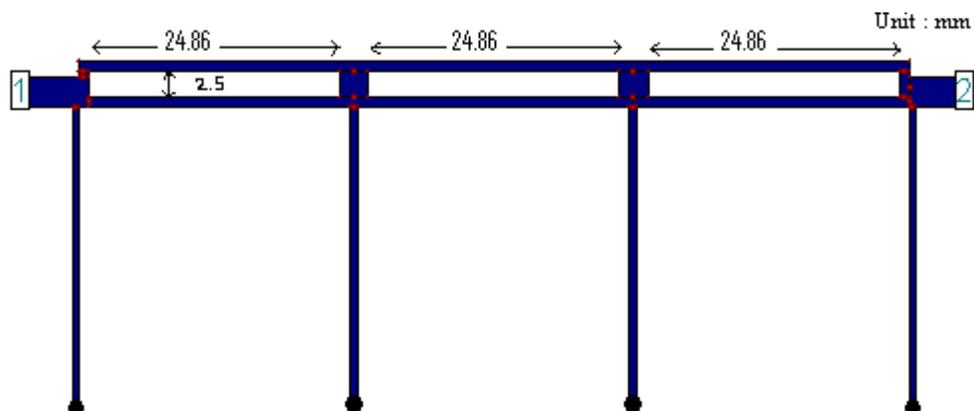
Figure 9. Layout of the etched UWB band pass filter.
