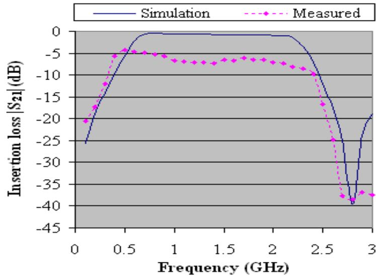
Figure 7. Comparison plot of insertion loss of the UWB Band pass filter
