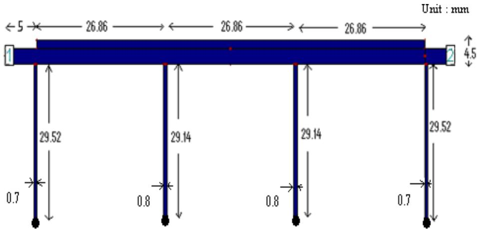
Figure 5. Microstrip UWB band pass filter using four Short-circuited stubs.
