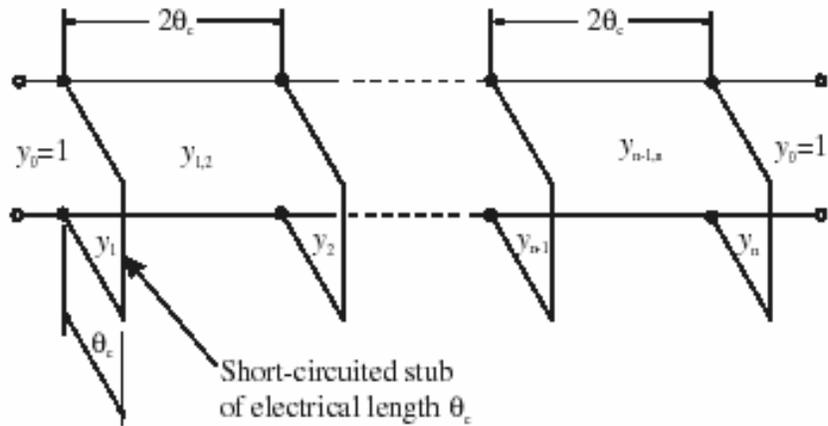
Figure 1. General circuit model for distributed UWB Band pass filter.
