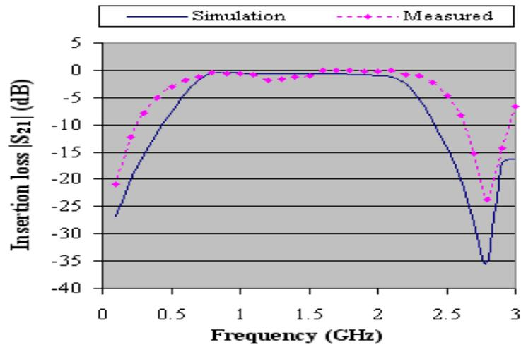
Figure 11. Comparison plot of insertion loss for the etched UWB filter.
