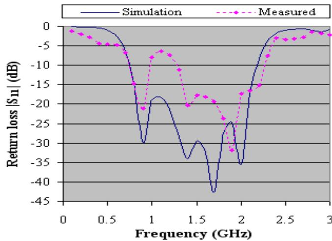
Figure 12. Comparison plot of return loss for the etched UWB filter.
