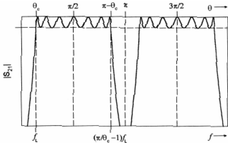
Figure 2. Typical filtering characteristics of the distributed UWB Band pass filter.
