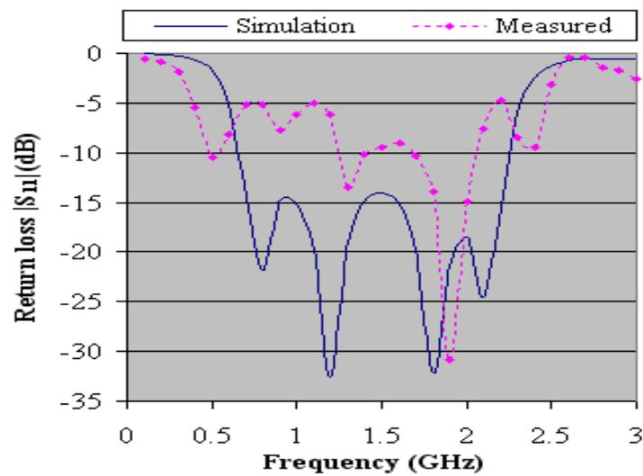
Figure 8. Comparison plot of return loss of the UWB Band pass filter.
