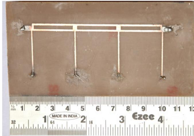
Figure 10. Fabricated layout of the etched UWB band pass filter.
