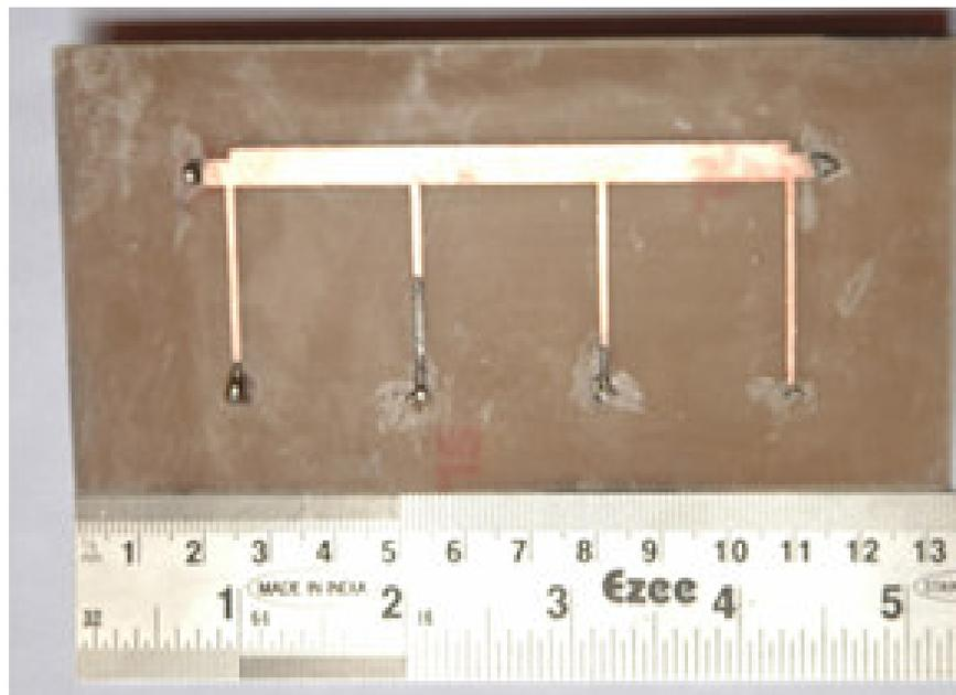
Figure 6. Photographed layout of the UWB band pass filter with via-hole grounding.
