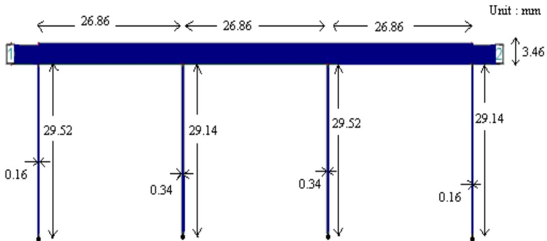
**Figure 3.** Microstrip Distributed UWB band pass filter using four Short-circuited stubs.
