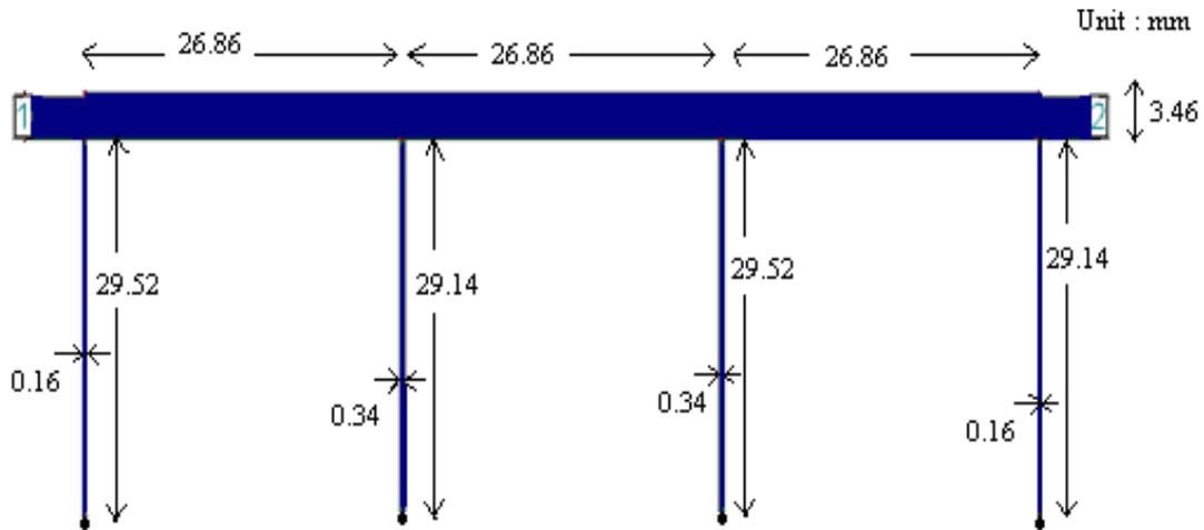
**Figure 3.** Microstrip Distributed UWB band pass filter using four Short-circuited stubs.
