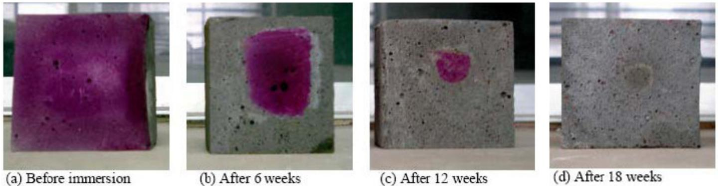
**Figure 1.** Residual alkalinity in 10% acid sulfuric solution.
