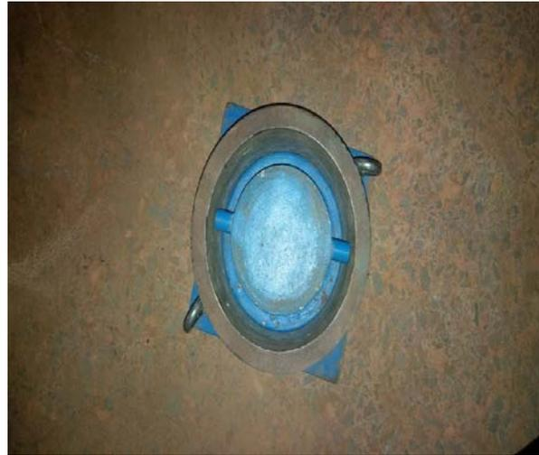
Plate 3. Apparatus for aggregate crushing test.
