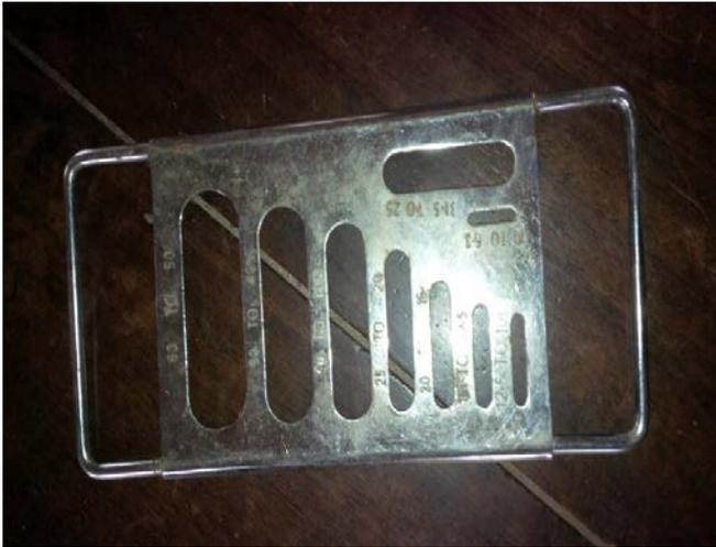
**Plate 4.** Thickness gauge for flakiness index determination.
