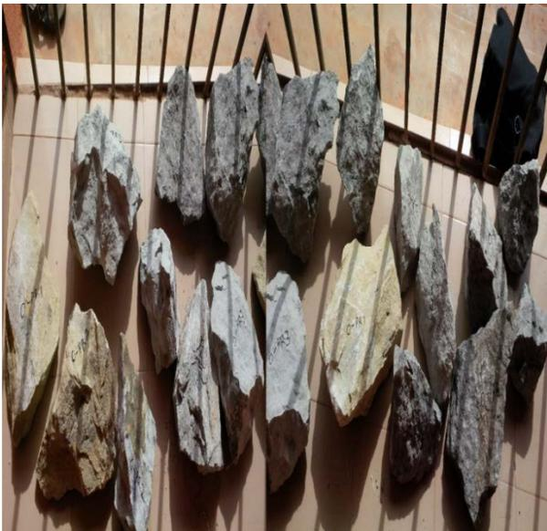
**Plate 5.** Sandstone lumps for aggregate.
