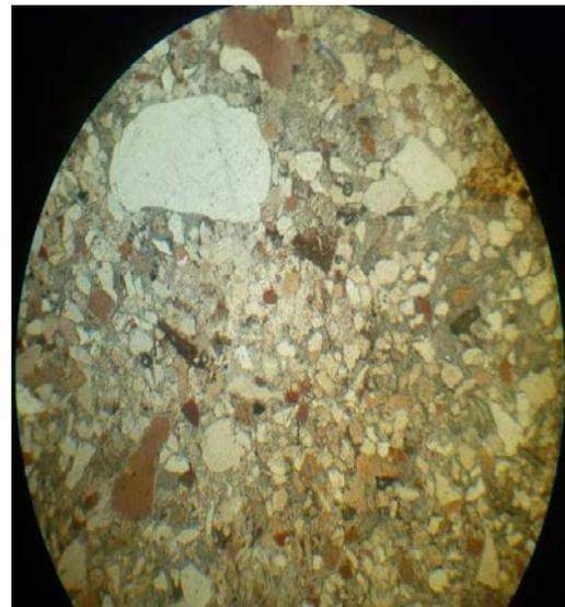
**Plate 7.** Convex to line contact, monocrystalline quartz, angular to subangular grain, moderately sorted.
