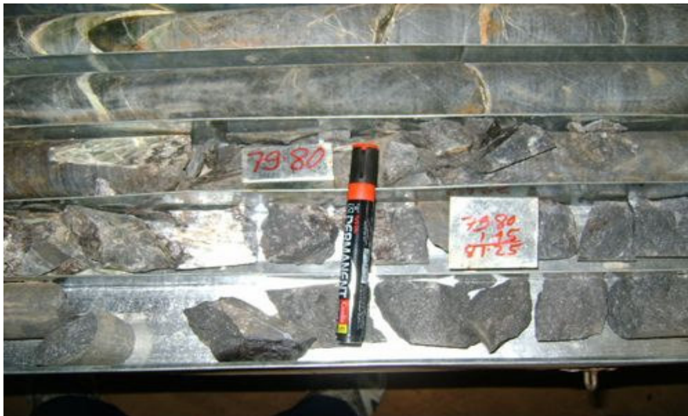
Figure 4. Core box showing chromitite at depth of 79.80 m.
