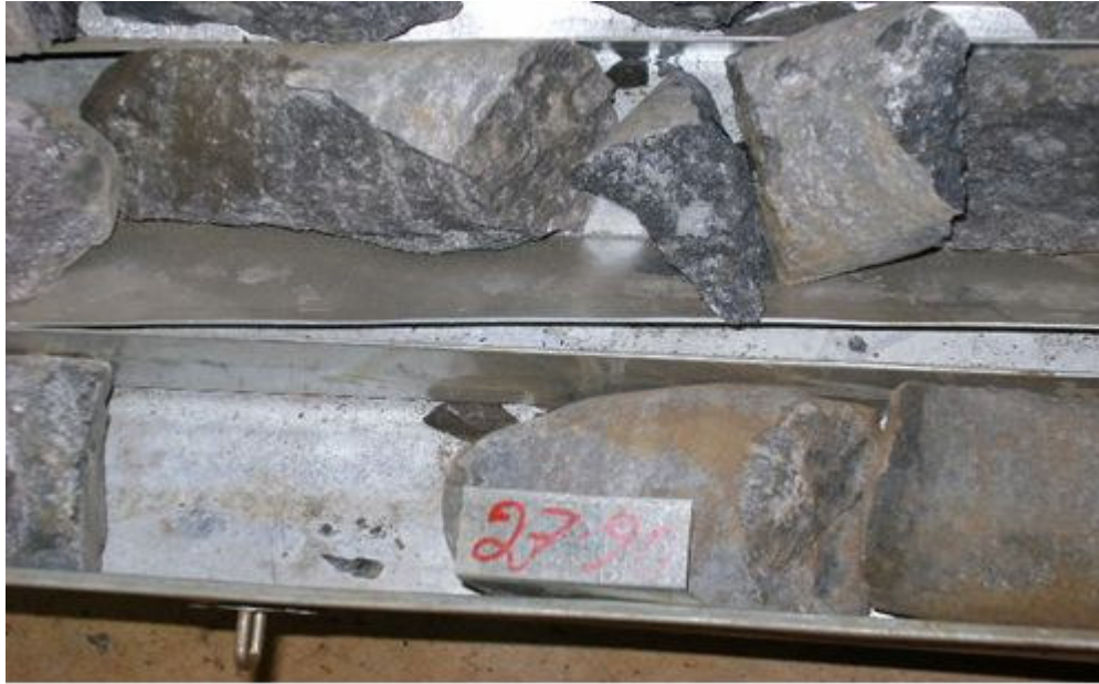
Figure 3. Core box showing chromitite at depth of 27.90 m.
